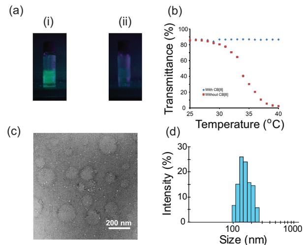
**Fig. 3** (a) Photographs showing the effect of addition of CB[8] to a solution of **1** + **2** (i) without CB[8] and (ii) with CB[8]. The formation of supramolecular ternary complexes leads to quenching of the pyrene fluorescence (excitation at 303 nm). (b) Thermoresponsive behaviour of **1** + **2** with and without CB[8] (0.05 mM). (c) TEM micrographs of supramolecular micelles at 37 °C (solution concentration = 0.05 mM). (d) Particle size distributions of supramolecular vesicles at 37 °C.
