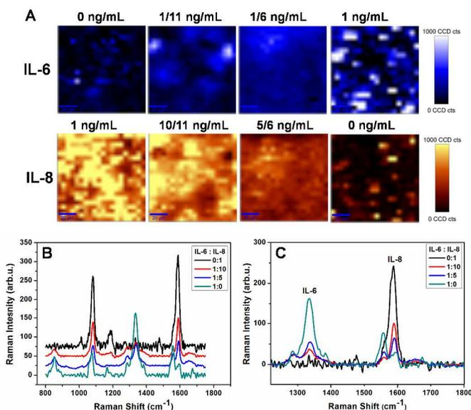
**Fig. 4.** Typical false-color SERS images (A) for duplex cytokine detection. The total protein amount was kept constant, but the IL-6/IL-8 ratio was varied from 0:1, 1:10, 1:5 to 1:0. Average SERS spectra (B and C) were determined from the corresponding SERS microspectroscopic data.
