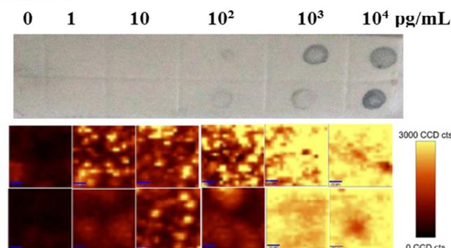
**Fig. 2.** Wide-field optical images of the SERS dots (top) and representative false-color SERS images for IL-6 detection at different antigen concentrations (bottom).
