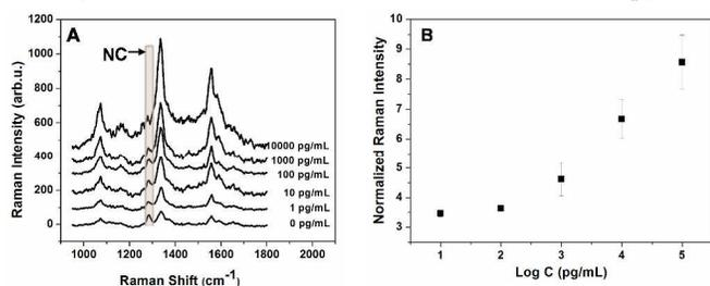
**Fig. 3.** Concentration-dependent average SERS spectra (A) and the corresponding concentration-dependent response function (from 1 pg/mL to 10 ng/mL) based on normalized SERS intensities (B) for the detection of IL-6.
