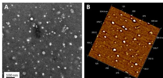
**Figure 2** Nanoassemblies incorporating DNJ-based glycopolymer **3**. A) TEM imaging; B) AFM imaging; C) Light-scattering analysis of the nanoparticles depending on the DNJ-based glycopolymer **3** content.
