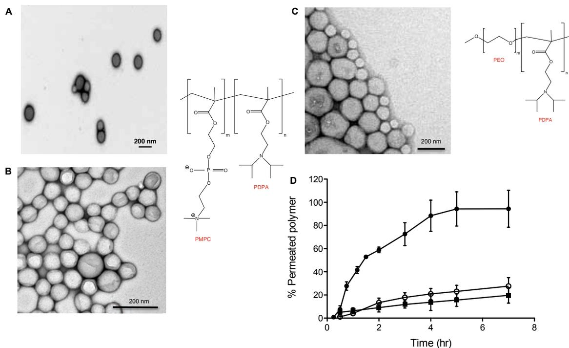
**Figure 2.** Polymersome formulations and relative permeations across a 50 nm pore sized membrane. (A) TEM micrograph and chemical structure of PMPC<sub>25</sub>-PDPA<sub>70</sub>. (B) TEM micrograph and chemical structure of PMPC<sub>25</sub>-PDPA<sub>500</sub>. (C) TEM micrograph and chemical structure of PEO<sub>113</sub>-PDPA<sub>70</sub>. (D) Permeation profiles as a function of time of
