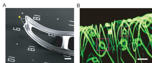
**Fig. 2** Flexible and three dimensional nanoelectronic devices. (A) Scanning electron microscopy image of a single kinked nanowire probe used for intracellular potential recording. The yellow star highlights the position of a field effect transistor. Scale bar, 5  $\mu\text{m}$ . (B) Confocal fluorescence microscopy image of a macroporous nanoelectronic scaffold used for sensing from engineered tissues. Magenta boxes demarcate two field effect transistor devices. Scale bar, 20  $\mu\text{m}$ .
