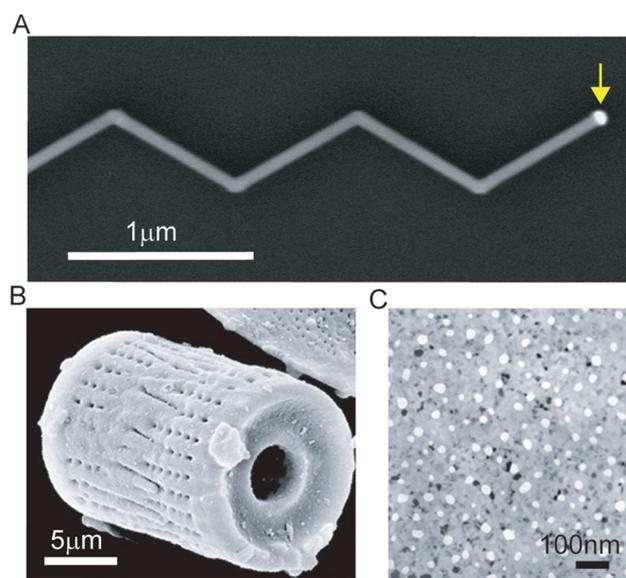
**Fig. 3** Complex silicon-based nanostructured materials. (A) Scanning electron microscopy image of a kinked nanowire; yellow arrow highlights the gold catalyst used for VLS growth. (B) A silicon 'diatom' synthesized by magnesium reduction. (C) A nanoporous silicon membrane used for molecular separation. B and C are adapted from ref. 51 and 52, respectively, with the permission from Nature Publishing Group.
