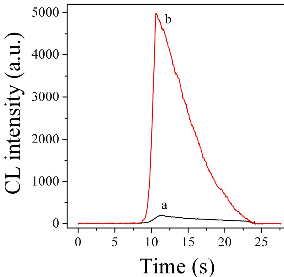
**Figure 2.** Kinetic curve of luminol-PIP-H<sub>2</sub>O<sub>2</sub> CL system: PBS (pH 7.4) in the absence (a) and presence of the 10.00  $\mu\text{L}$  6.00  $\mu\text{g mL}^{-1}$  of HRP-labeled goat anti-rabbit IgG (b), respectively. Conditions: 100.00  $\mu\text{L}$  of Tris-HCl (pH 8.5) containing 3.80 mM H<sub>2</sub>O<sub>2</sub>, 0.70 mM luminol and 0.60 mM PIP was injected.
