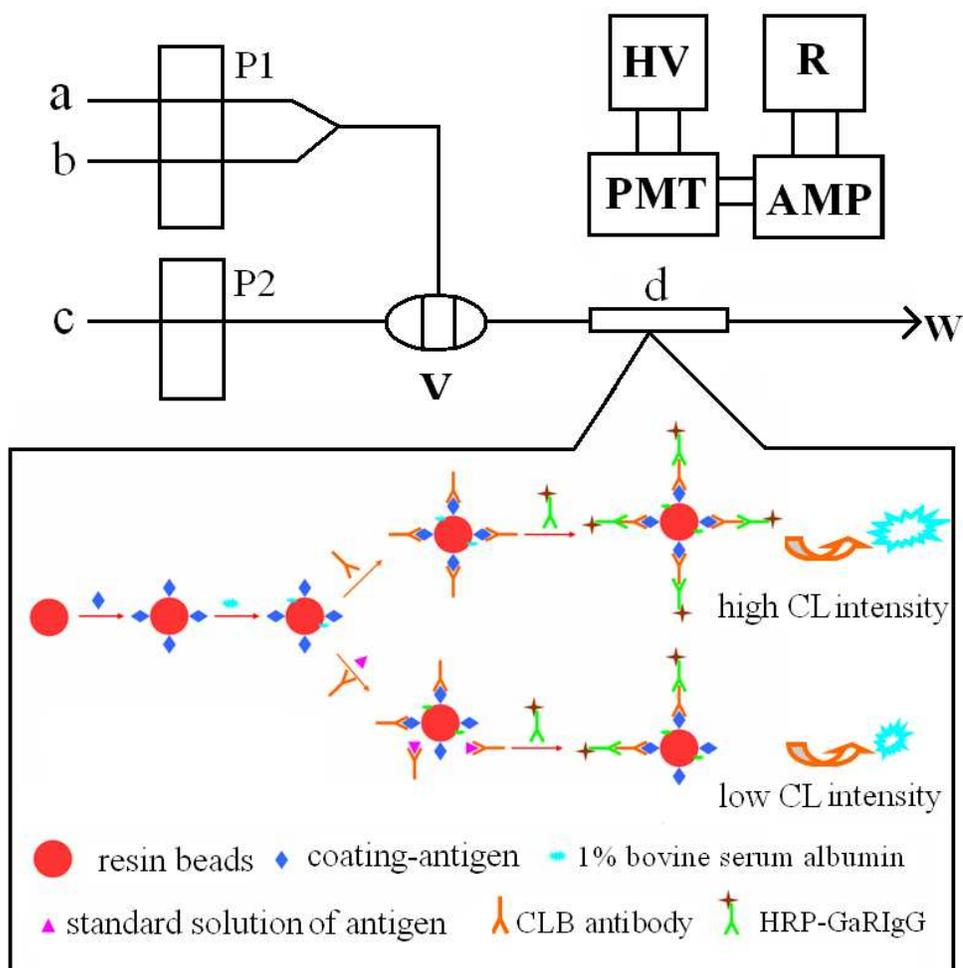
**Scheme 1.** Schematic diagram of the FIIA system manifold: (P1) peristaltic pump; (P2) syringe pump; (a) luminol and PIP; (b)  $\text{H}_2\text{O}_2$ ; (c) resin beads, sample, antibodies, washing buffer; (V) injection valve; (d) immunosensor; (PMT) photomultiplier; (HV) negative high voltage supply; (AMP) amplifier; (R) recorder; (W) waste.
