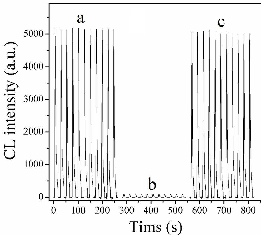
**Figure 5.** CL intensity of (a) a new assembled immunosensor flowing with CLB/Ab1+ HRP-GaRIgG, (b) the immunosensor washing with 0.1 M glycine-HCl (pH 2.2) and (c) the regenerative immunosensor injected into CLB/Ab1+ HRP-GaRIgG.
