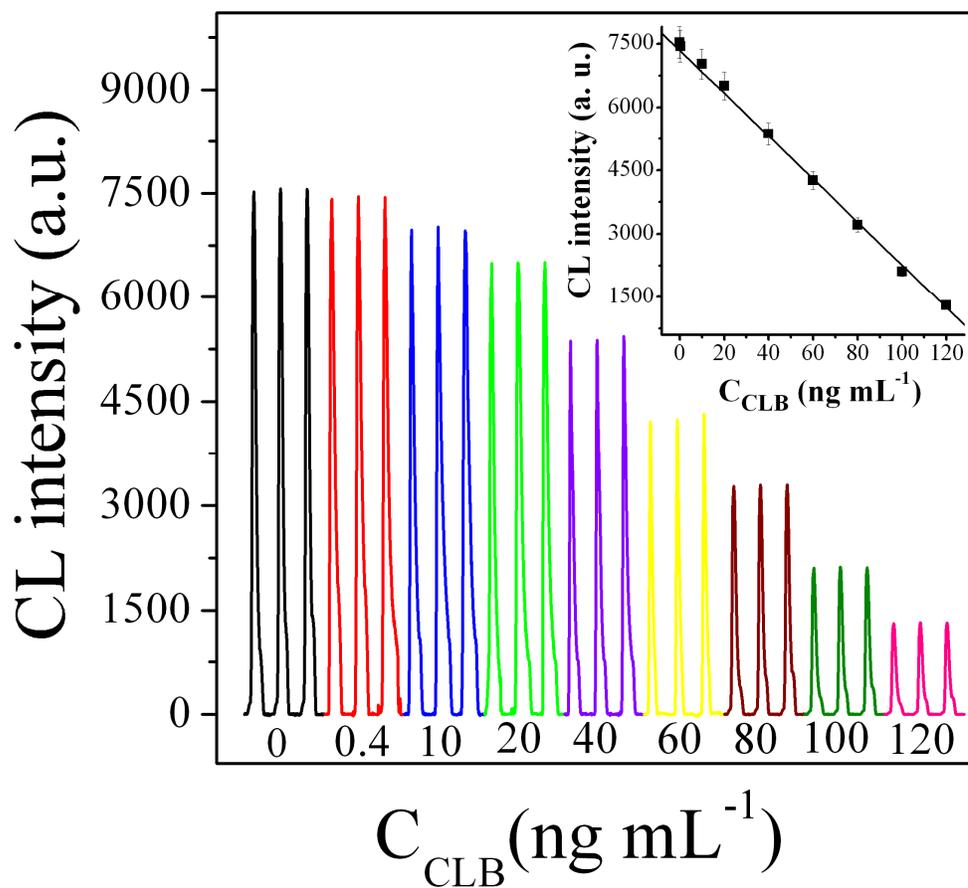
**Figure 4.** The CL responses of the immunosensor for detecting different concentrations of clenbuterol. Inset: calibration curve, where  $n = 5$  for each point. All the tests were performed under the optimal conditions.
