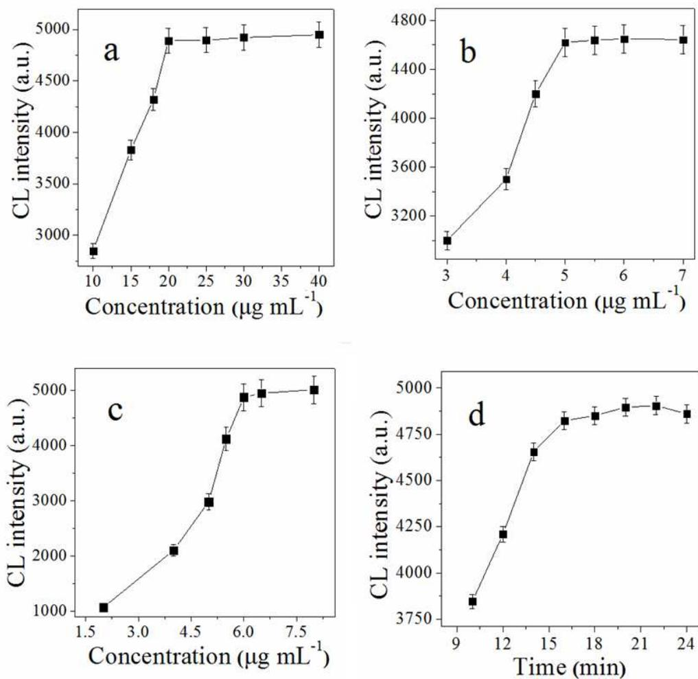
**Figure 3.** Effects of concentration of clenbuterol coating-antigen (a), clenbuterol antibody (b) and HRP-GaRIgG (c), and (d) pre-incubation time of clenbuterol and clenbuterol antibody on CL intensity.
