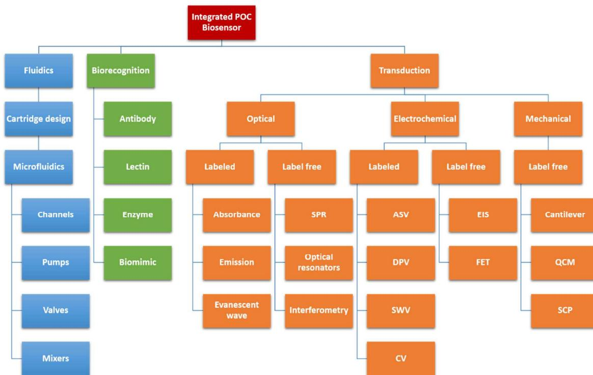
**Figure 5.** Main components of an integrated point-of-care biosensor.
