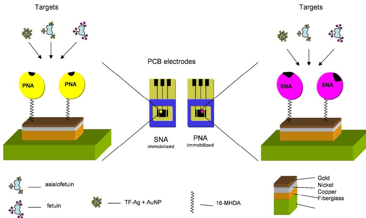
**Figure 6.** Label free EIS glycobiosensor. Printed circuit board (PCB) electrodes consisting of layered copper/nickel/gold films are covalently functionalized with either PNA or SNA lectins and probed with serial dilutions of TF-antigen encapsulated gold nanoparticles, asialofetuin (ASF) and fetuin (FET) resulting in 13-150fM limits of detection of TF-antigen.<sup>113</sup>
