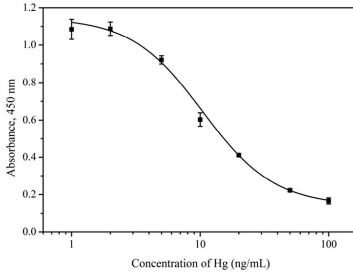
**Fig. 2** The standard inhibition curve for the Hg(II) indirect competitive ELISA
