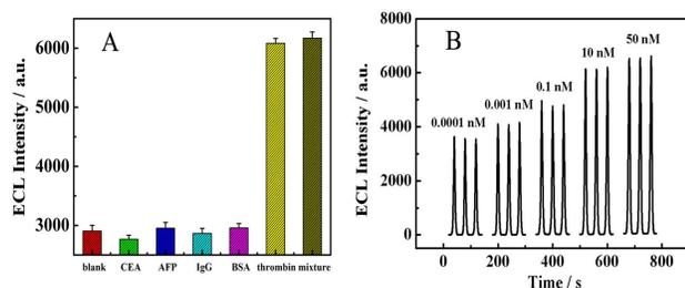
**Fig. 5** (A) Selectivity evaluation of the aptasensor against the interference molecules, CEA (100 nM), AFP (100 nM), IgG (100 nM), BSA (100 nM) and their mixing with TB. (B) ECL stability of proposed aptasensor with various concentrations of TB.
