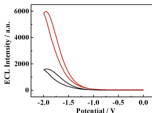
**Fig. 3** ECL intensity-potential curves of TBA II/TB/BSA/TBA /dep-Au modified GCE in 0.1 M peroxydisulfate in the absence (black curve) and in the presence of (red curve) 0.01 M glucose and 120  $\mu\text{L}$   $\text{NAD}^+$  (0.25 mM).
