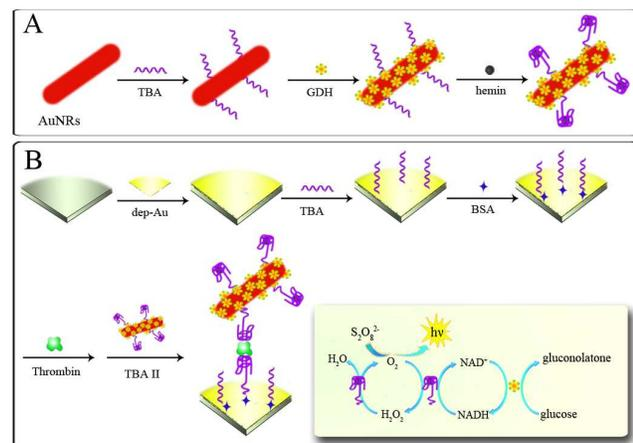
**Scheme 1** (A) The preparation procedure of secondary aptamer, (B) Schematic diagram of preparation and reaction mechanism of the ECL aptasensor.
