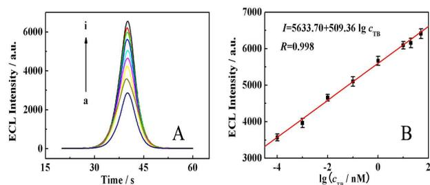
**Fig. 4** (A) ECL profiles of the proposed aptasensor to different concentrations of TB (a–i). (B) calibration curve for TB determination. The concentrations of TB: (a) 0 nM, (b) 0.0001 nM, (c) 0.001 nM, (d) 0.01 nM, (e) 0.1 nM, (f) 1.0 nM, (g) 10 nM, (h) 20 nM, (i) 50 nM. All ECL signals were measured in 2 mL PBS (pH 7.4) with 0.1 M peroxydisulfate, 0.01 M glucose and 120  $\mu$ L NAD<sup>+</sup> (0.25 mM).
