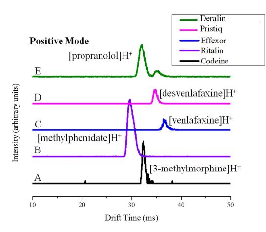
Figure 3. Positive DESI-IMS-TOFMS Drug Standard Data. The calculated  $K_o$  values for (A) Codeine ([3-methylmorphine]H<sup>+</sup>), (B) Ritalin ([methylphenidate]H<sup>+</sup>), (C) Effexor ([venlafaxine]H<sup>+</sup>), (D) Pristiq ([desvenlafaxine]H<sup>+</sup>) and (E) Deralin ([R/S-propranolol]H<sup>+</sup>) were 1.30, 1.46, 1.22, 1.17 and 1.26 cm<sup>2</sup>/Vs, respectively.
