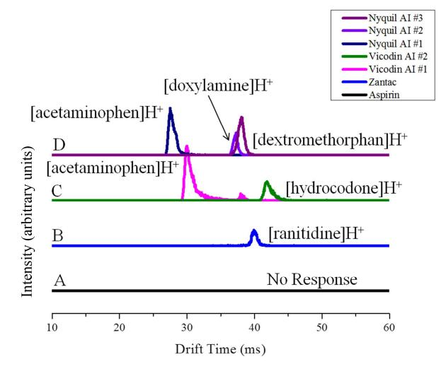
*Figure 4. Positive Mode DESI-IMS-TOFMS Sample Drug Data.* The calculated  $K_o$  values for (*B*) Zantac ([ranitidine] $H^+$ ), (*C*) Vicodin active ingredient #1 ([acetaminophen] $H^+$ ), (*D*) Vicodin active ingredient #2 ([hydrocodone] $H^+$ ), Nyquil active ingredient #1 ([acetaminophen] $H^+$ ), Nyquil active ingredient #2 ([doxylamine] $H^+$ ) and Nyquil active ingredient #3([dextromethorphan] $H^+$ ) were 1.07, 1.41, 1.02, 1.41, 1.15 and 1.12 cm<sup>2</sup>/Vs, respectively.
