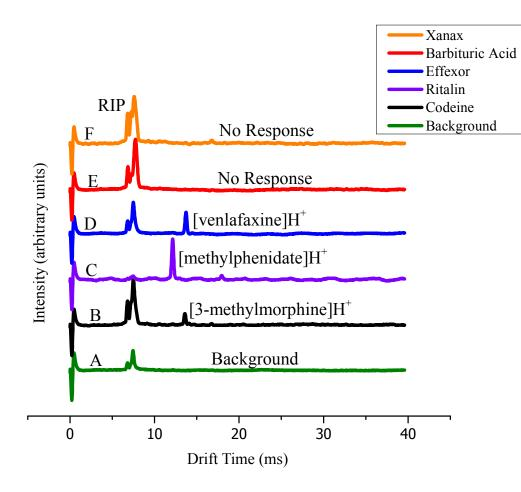
Figure 2. Positive Mode Standalone DESI-IMS Drug Standard Data The calculated  $K_o$  values for (**B**) Codeine ([3-methylmorphine] $H^+$ ), (**C**) Ritalin ([methylphenidate] $H^+$ ) and (**D**) Effexor ([venlafaxine] $H^+$ ) were 1.27, 1.43 and 1.26 cm<sup>2</sup>/Vs ( $\pm 0.01$ cm<sup>2</sup>/Vs), respectively. (**E**) Barbituric acid and (**F**) Xanax were not detected in the positive mode.
