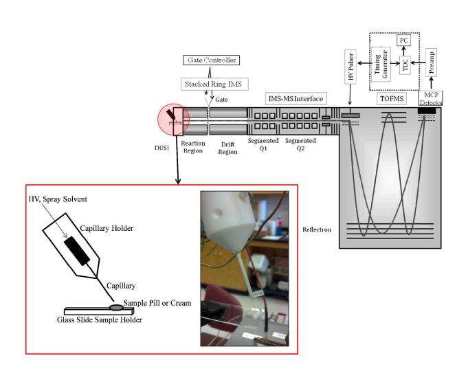
**Figure 1. IM-TOFMS Instrument Schematic.** Pictured from left to right is the DESI source, ion mobility spectrometer, IMS-MS interface (segmented Q1, segmented Q2 and lens region), TOF mass spectrometer and MCP detector. Insert shows DESI schematic and photograph of set
