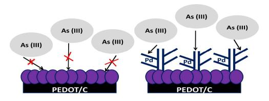
**Scheme 1:** Schematic representation of As(III) ions adsorbed on the surface of Pd nanodendrities on PEDOT coated carbon paper.
