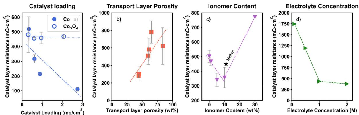
Fig. 4 Impact of (a) Co and  $Co_3O_4$  catalyst loading, (b) PTL porosity, (c) the ionomer content/type, and (d) the KOH supporting electrolyte concentration on  $R_{CL}$ . All results are for changes in the anode catalyst layer only. Dashed lines are guides for the eye. In (a)–(c), the average and standard deviations of three experiments are plotted as the markers and error bars, respectively.
