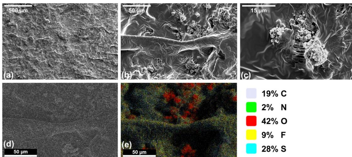
Fig. 8 SEM images of Li anode of the Li-S EL-Cell with 600  $\mu\text{m}$  electrolyte thickness in post mortem analysis. Three different magnifications of (a)  $\times 200$ , (b)  $\times 2000$ , (c)  $\times 8000$ , and (d) and (e) element mapping obtained *via* EDX analysis.
