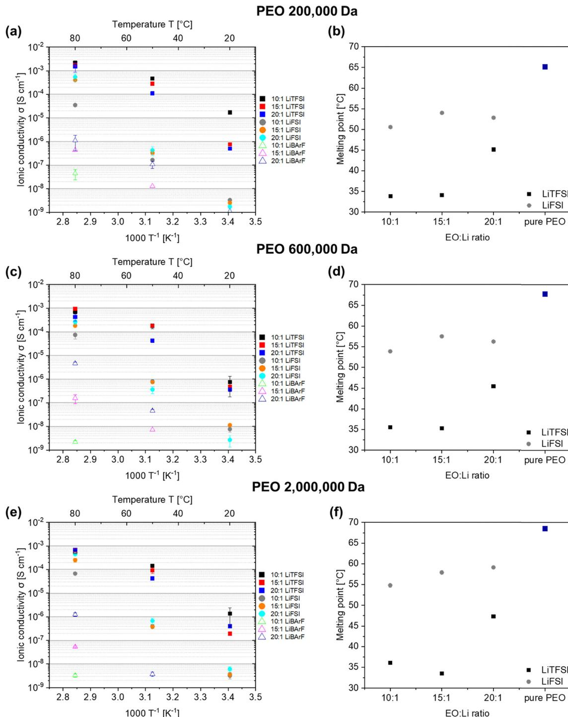
Fig. 2 Evaluation of the ionic conductivity as determined by EIS (a), (c) and (e) and the melting point obtained *via* DSC (b), (d) and (f) of the solid electrolyte films with different conducting salts (LiTFSI, LiFSI, LiBARf), Li salt concentrations (EO : Li ratio) and PEO molecular weights of 200 000, 600 000 and 2000 000 Da.
