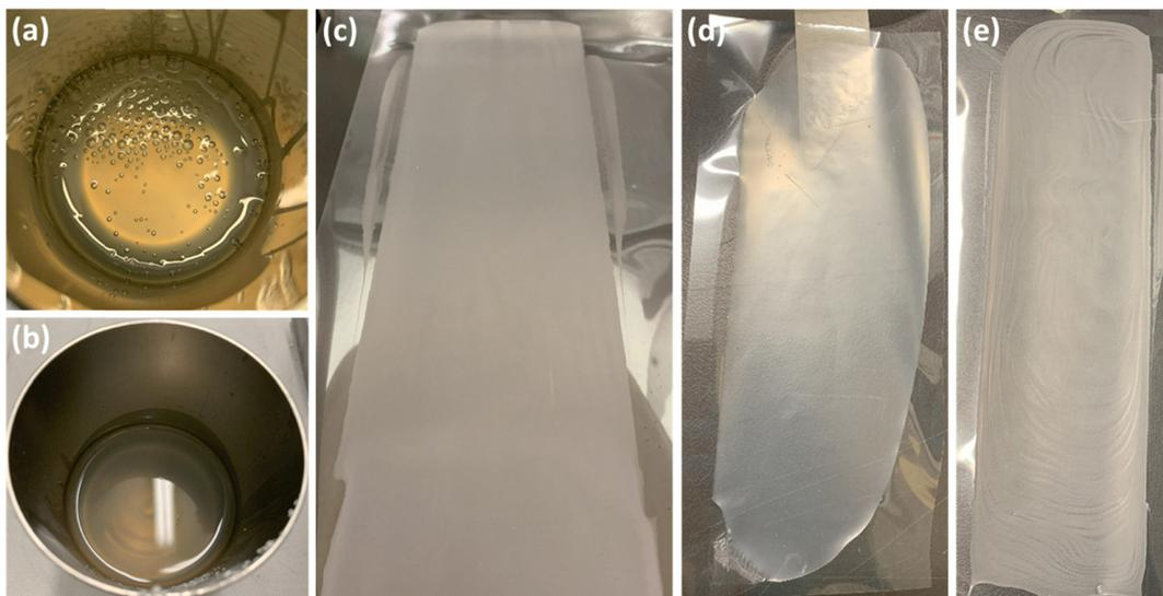
**Fig. 1** Representative examples for solvent-based solid electrolyte film production. (a) Electrolyte solution with air bubbles and (b) after vacuum treatment. Solid electrolyte film on transparent substrate foil with (c) lithium bis(trifluoromethylsulfonyl)amide (LiTFSI), (d) lithium bis(fluorosulfonyl)imide (LiFSI) and (e) lithium tetrakis(pentafluorophenyl)borate (LiBARF).
