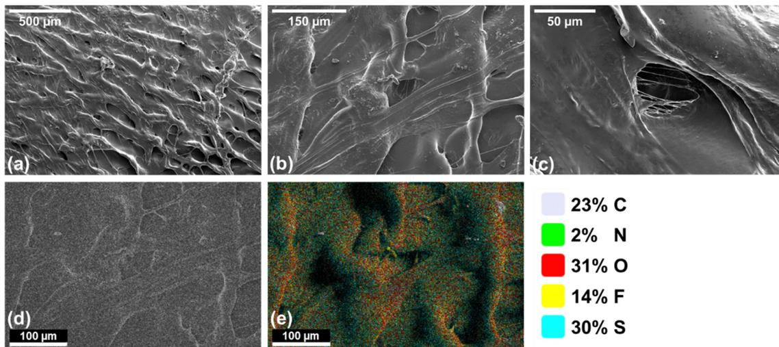
Fig. 9 SEM images of the sulfur cathode of the Li-S EL-cell with 600  $\mu\text{m}$  electrolyte thickness in post-mortem analysis. Three different magnifications of (a)  $\times 200$ , (b)  $\times 800$ , (c)  $\times 2000$  and (d) and (e) element mapping obtained from EDX analysis.
