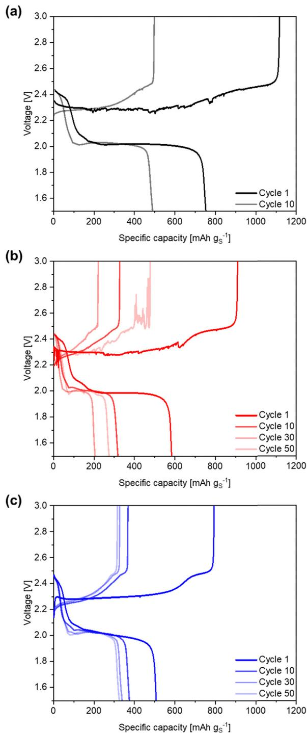
Fig. 6 Voltage-capacity profiles for the cycled Li-S EL-cells with different electrolyte thickness of (a) 150  $\mu\text{m}$ , (b) 300  $\mu\text{m}$ , and (c) 600  $\mu\text{m}$ .
