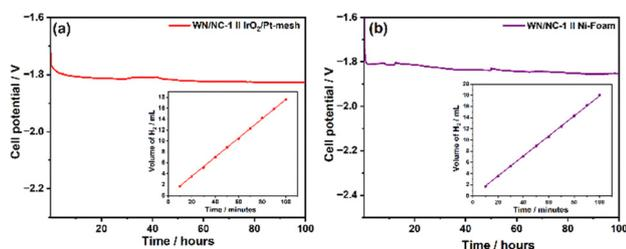
Fig. 6 Chronopotentiometry curves of WN/NC-1-coated cathode water electrolyzers: (a) 0.5 M H<sub>2</sub>SO<sub>4</sub> (PEM) and (b) 1 M KOH (AEM) electrolytes at the constant current density of 10 mA cm<sup>-2</sup>. The insets indicate the quantity of hydrogen evolved from the cathodes with time.
