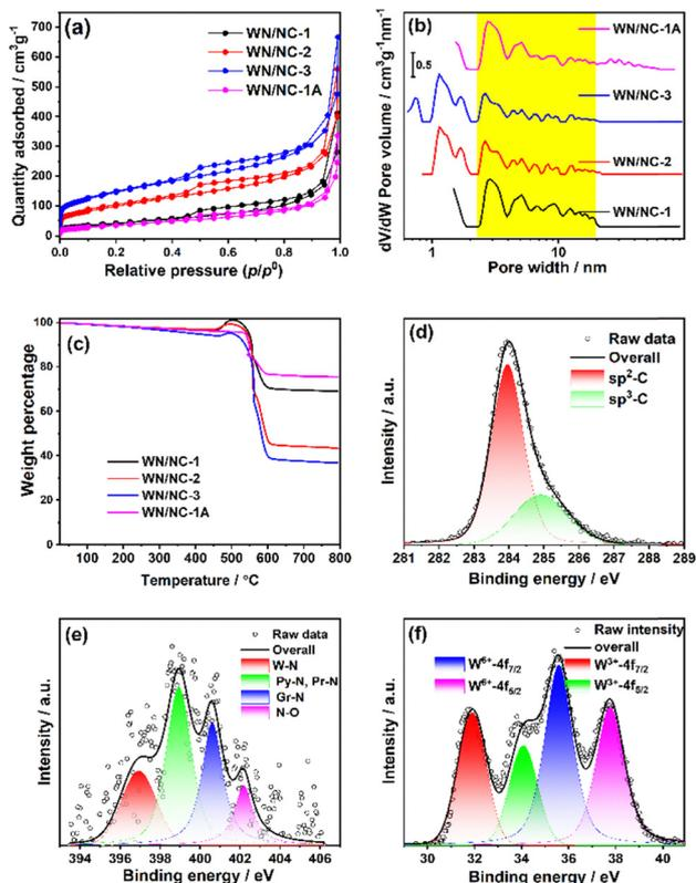
Fig. 3 (a) The  $N_2$ -sorption isotherms of the WN/NC catalysts and (b) their NLDFT pore size distribution plot. (c) Thermogravimetric plots of the WN/NC catalysts in an air atmosphere. The (d) C-1s, (e) N-1s and (f) W-4f XPS of WN/NC-1 and their deconvoluted peaks.
