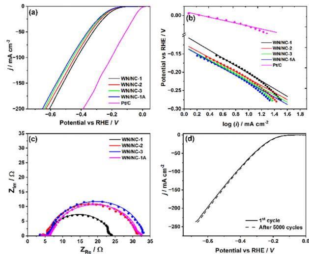
Fig. 4 Linear sweep voltammogram of the WN/NC catalysts in  $N_2$ -saturated 0.5 M  $H_2SO_4$  electrolyte at a scan rate of  $5 \text{ mV s}^{-1}$  and 1600 rotational speed, and the (b) Tafel plots, (c) electrochemical impedance spectroscopy analysis of the WN/NC catalysts at an overpotential of 190 mV and (d) linear sweep voltammogram of the HER on the WN/NC-1 catalyst before and after 5000 cycles of accelerated durability test (ADT).
