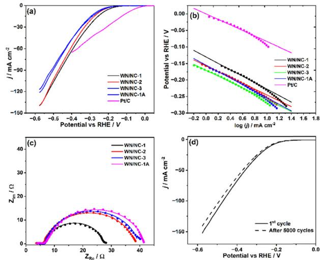
Fig. 5 (a) Linear sweep voltammogram of the WN/NC catalysts in  $\text{N}_2$ -saturated  $1 \text{M KOH}$  as the electrolyte, (b) its Tafel plots, (c) electrochemical impedance spectroscopy analysis of the WN/NC catalysts at an overpotential of  $200 \text{mV}$  and (d) linear sweep voltammogram of the WN/NC-1 catalyst before and after 5000 cycles of accelerated durability test (ADT).
