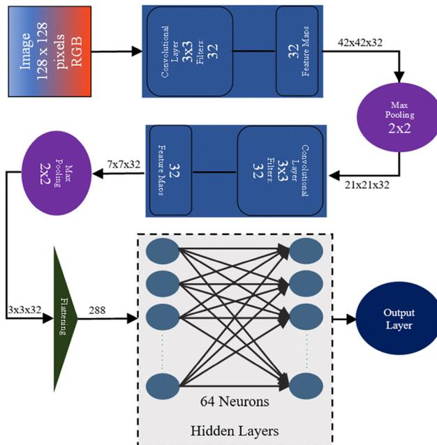
Fig. 3 The convolutional neural network (CNN) architecture employed in this work.
