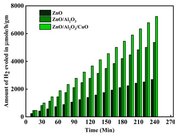
Fig. 12 H<sub>2</sub> evolution rate *via* water splitting using ZnO and ZnO/Al<sub>2</sub>O<sub>3</sub> and ZnO/Al<sub>2</sub>O<sub>3</sub>/CuO nanocomposite.
