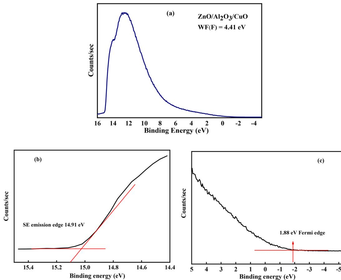
Fig. 10 (a) UPS spectra of the ZnO/Al<sub>2</sub>O<sub>3</sub>/CuO nanocomposite film showing (b) the secondary edge at high binding energy region related to work function and (c) the low energy region related to valence band maximum.
