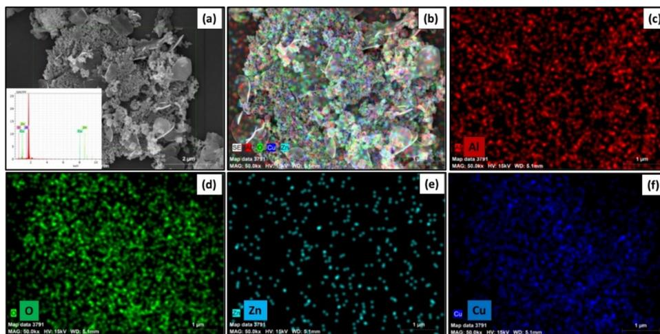
Fig. 4 Elemental mapping of the ZnO/Al<sub>2</sub>O<sub>3</sub>/CuO nanocomposite: (a) FE-SEM with EDS, (b) overlapped elemental map, (c) Al elemental map, (d) O elemental map, (e) Zn elemental map, and (f) Cu elemental map.
