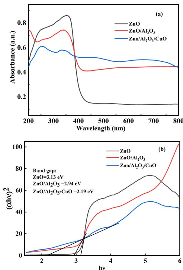
Fig. 1 (a) UV-Visible spectra and (b) Tauc plot of ZnO, ZnO/Al<sub>2</sub>O<sub>3</sub> and ZnO/Al<sub>2</sub>O<sub>3</sub>/CuO nanocomposite.
