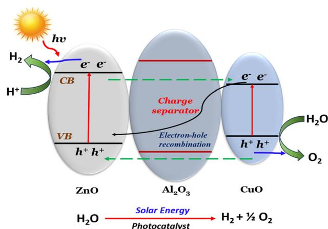
**Fig. 13** Plausible Z-scheme photocatalytic mechanism illustrating charge transfer in the ZnO/Al<sub>2</sub>O<sub>3</sub>/CuO heterojunction for simultaneous hydrogen and oxygen evolution under solar irradiation.
