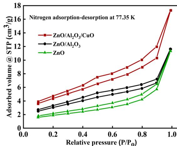
Fig. 7 BET curves of ZnO, ZnO/Al<sub>2</sub>O<sub>3</sub>, and ZnO/Al<sub>2</sub>O<sub>3</sub>/CuO nanocomposite.
