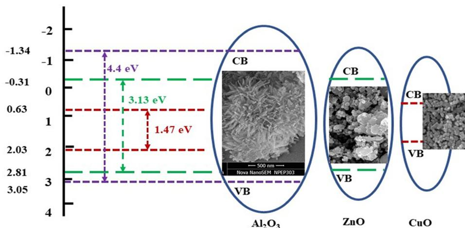
Fig. 9 Schematic diagrams representing energy bands of ZnO/Al<sub>2</sub>O<sub>3</sub>/CuO nanocomposite.
