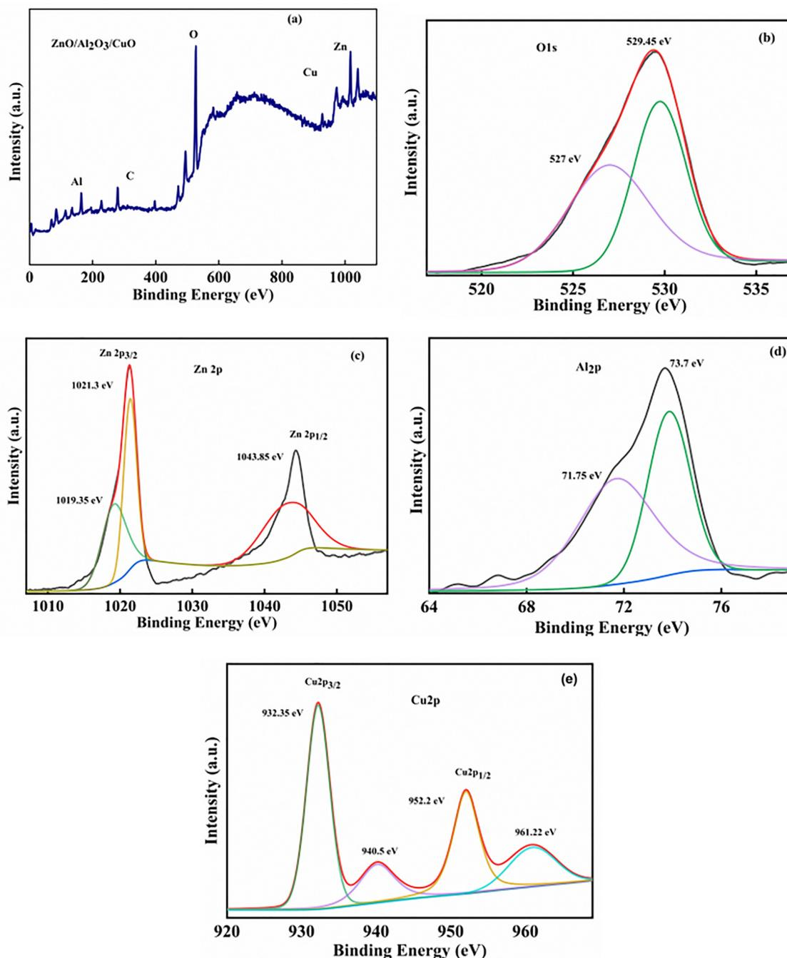
Fig. 8 (a) Survey scan of ZnO/Al<sub>2</sub>O<sub>3</sub>/CuO nanocomposite, and high resolution XPS spectra of the core level of (b) O 1s, (c) Zn 2p, (d) Al 2p and (e) Cu 2p.
