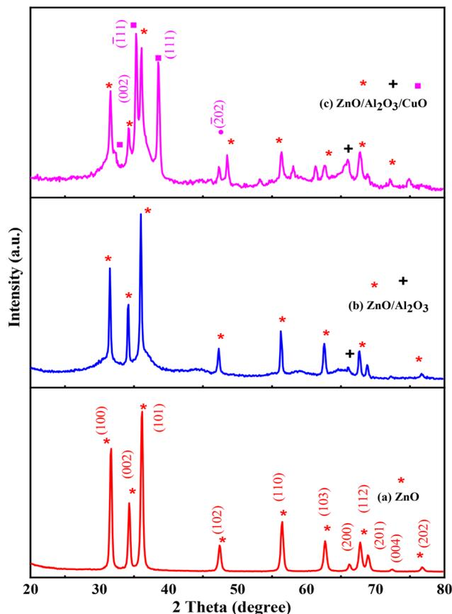
Fig. 2 X-Ray diffraction patterns of (a) ZnO, (b) ZnO/Al<sub>2</sub>O<sub>3</sub>, and (c) ZnO/Al<sub>2</sub>O<sub>3</sub>/CuO nanocomposite.
