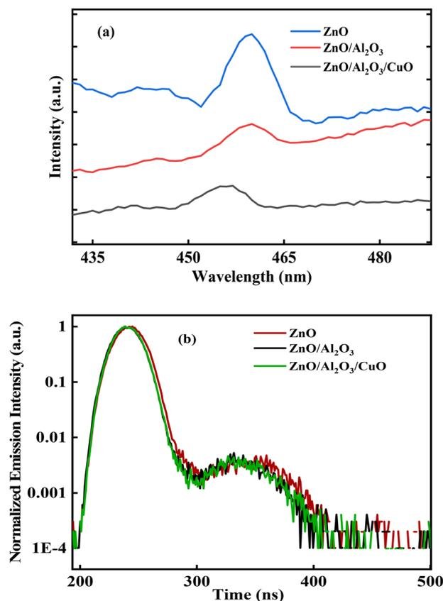
Fig. 11 (a) Photoluminescence (PL) spectra and (b) Time-resolved photoluminescence (TRPL) spectra of ZnO, ZnO/Al<sub>2</sub>O<sub>3</sub>, and ZnO/Al<sub>2</sub>O<sub>3</sub>/CuO nanocomposites.
