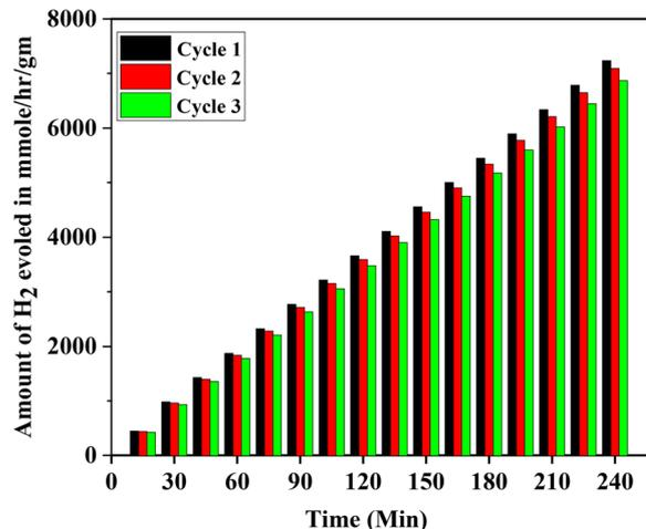
Fig. 14 Photocatalytic hydrogen evolution stability of the ZnO/Al<sub>2</sub>O<sub>3</sub>/CuO nanocomposite over three consecutive cycles under identical reaction conditions.
