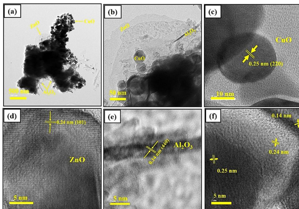
Fig. 5 (a) and (b) TEM images for ZnO/Al<sub>2</sub>O<sub>3</sub>/CuO nanocomposite, (c)–(f) HRTEM image for CuO, ZnO, Al<sub>2</sub>O<sub>3</sub> in nanocomposite respectively.
