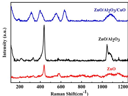
Fig. 6 Raman spectrum of ZnO, ZnO/Al<sub>2</sub>O<sub>3</sub> and ZnO/Al<sub>2</sub>O<sub>3</sub>/CuO nanocomposite.
