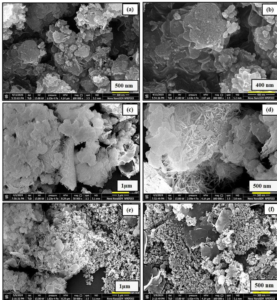
Fig. 3 FESEM Micrograph for ZnO (a), (b), ZnO/Al<sub>2</sub>O<sub>3</sub> (c), (d), and ZnO/Al<sub>2</sub>O<sub>3</sub>/CuO nanocomposite (e), (f).
