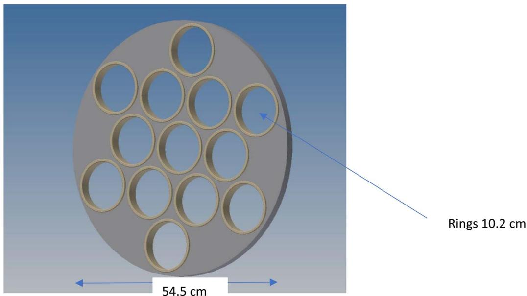
Fig. 2 Schematic of the floating microcosm (not drawn to scale with a diameter of 54.5 cm and inner rings of 10.2 cm diameter).
