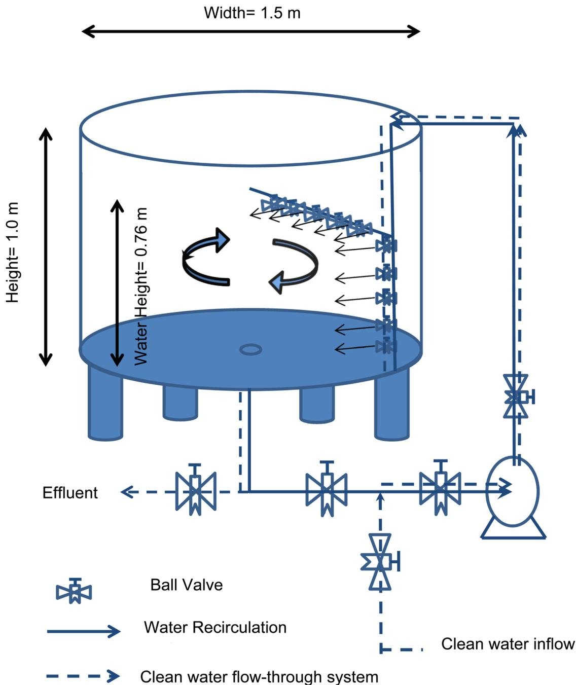
Fig. 1 Schematic of the circular flume tank (not drawn to scale).
