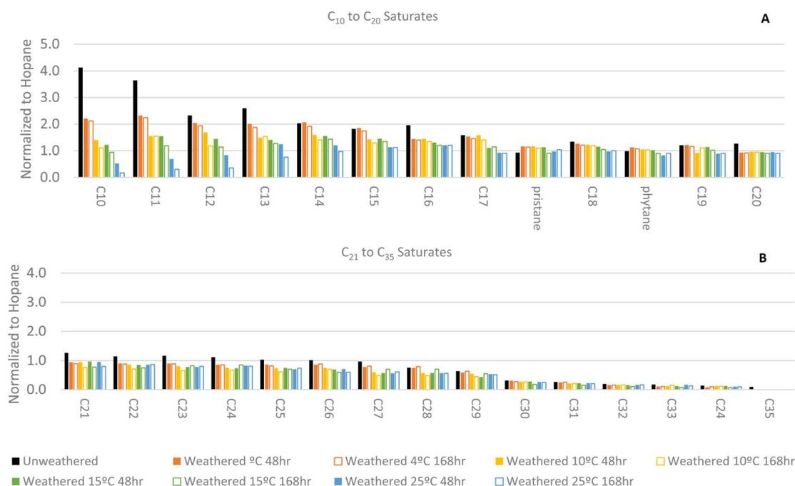
Fig. 5 A plot of the decrease in saturates (A) C<sub>10</sub> to C<sub>20</sub> and (B) C<sub>21</sub> to C<sub>35</sub> of Cold Lake Blend (CLB) diluted bitumen composite samples over a range of temperatures at 48 and 168 hours of weathering on sea water.  $T = 0$  represents unweathered oil.
