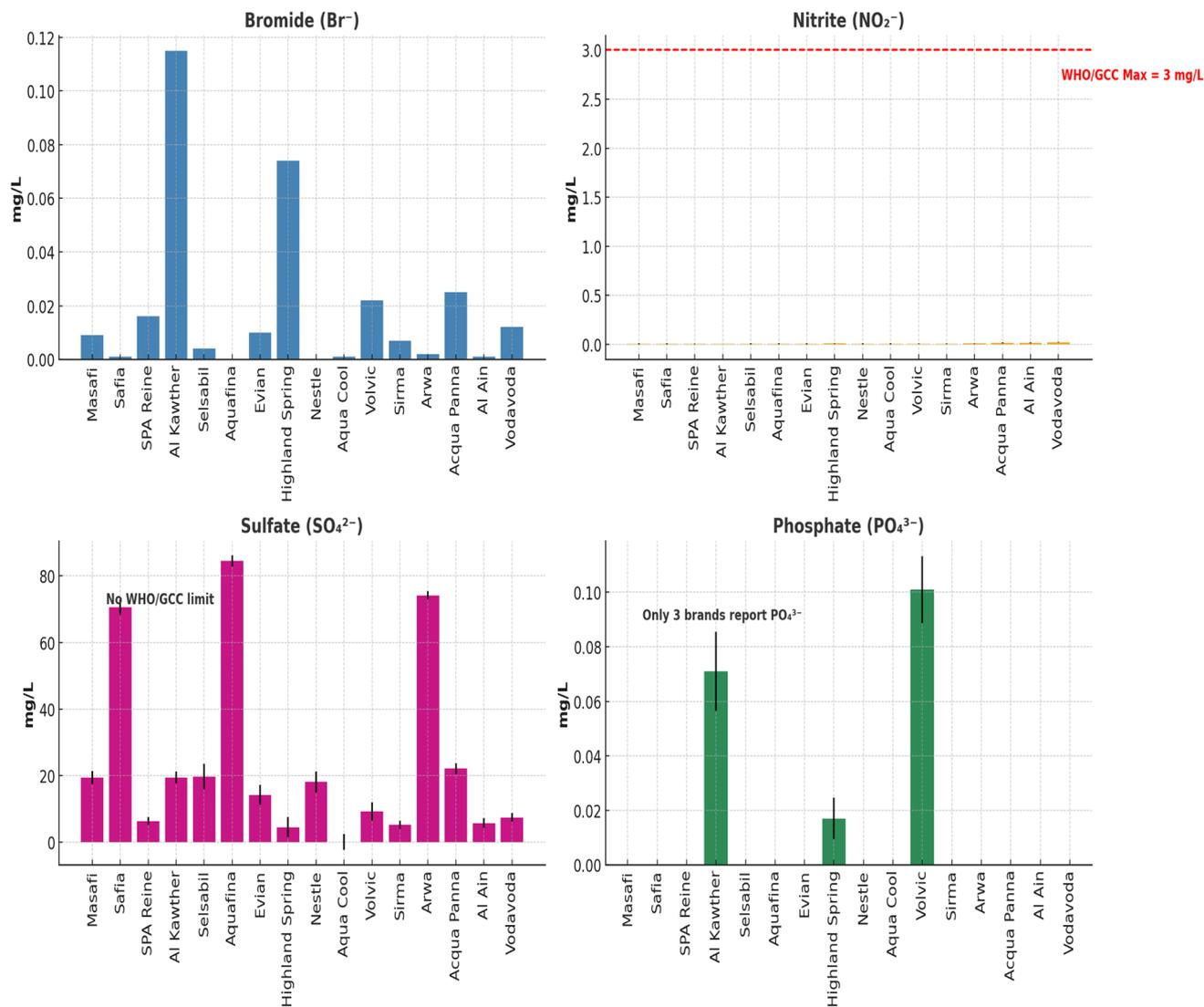
Fig. 4 Concentrations of additional anions ( $\text{Br}^-$ ,  $\text{NO}_2^-$ ,  $\text{SO}_4^{2-}$ ,  $\text{PO}_4^{3-}$ ) in bottled water. Phosphate data were only available for three brands. WHO/GCC guideline lines are shown for  $\text{NO}_2^-$ ; no limits exist for  $\text{SO}_4^{2-}$  or  $\text{Br}^-$ .
