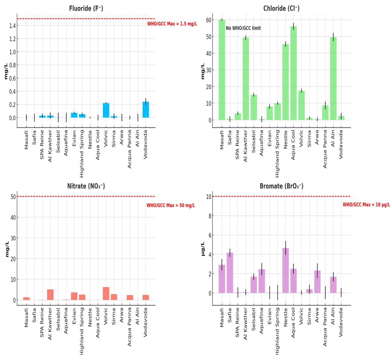
Fig. 3 Concentrations of major anions ( $\text{F}^-$ ,  $\text{Cl}^-$ ,  $\text{NO}_3^-$ ,  $\text{BrO}_3^-$ ) in bottled water samples. Error bars represent estimated standard deviations from replicate analyses. WHO/GCC guideline thresholds are annotated where applicable.
