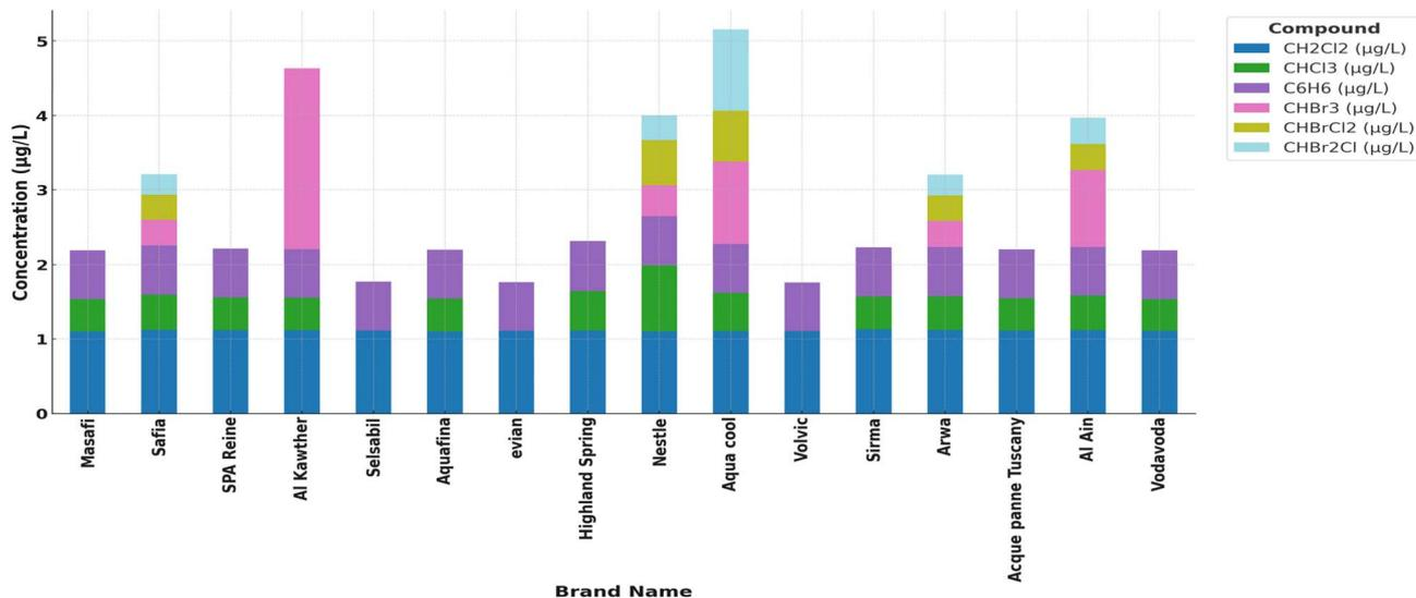
Fig. 7 Concentration and compound-specific distribution of Trihalomethanes (THMs) and volatile organic compounds (VOCs) detected in bottled water brands. The chart displays six key analytes: CH<sub>2</sub>Cl<sub>2</sub> (dichloromethane), CHCl<sub>3</sub> (chloroform), C<sub>6</sub>H<sub>6</sub> (benzene), CHBr<sub>3</sub> (bromoform), CHBrCl<sub>2</sub> (dibromochloromethane), and CHBr<sub>2</sub>Cl (bromodichloromethane). Stacked columns reflect the cumulative THM/VOC load per brand.
