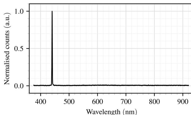
Fig. 2 Normalised spectrum of the laser diode.
