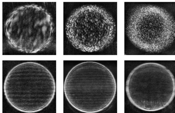
**Fig. 9** Defocused images of PP particles (top) and air bubbles (bottom). Particle size increases from left to right, as indicated by the change in fringe and speckle structure rather than by the apparent image diameter. Images were cropped to the particle and contrast enhanced to improve clarity.
