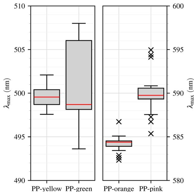
Fig. 6 Wavelengths of the emission maxima ( $\lambda_{\max}$ ) of fluorescence spectra from PP particles with different fluorescent dyes. Boxplots display the distribution of  $\lambda_{\max}$  values, indicating median, interquartile range, whiskers, and outliers for each sample.
