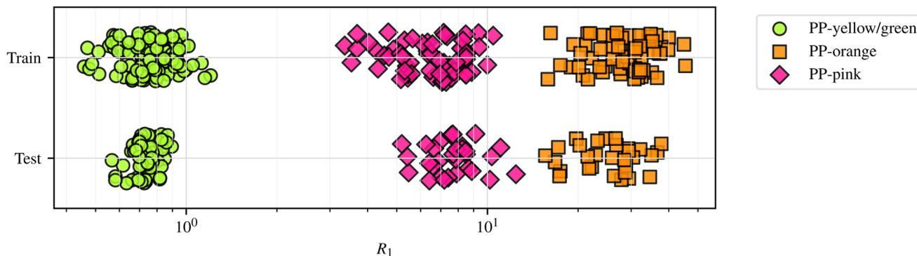
Fig. 7 Train and test values of  $R_1$  for PP samples with different fluorescent dyes. Each point corresponds to one particle; colours denote fluorescent dyes (yellow/green, orange, pink). The upper row shows the training data, while the lower row displays the corresponding test data.
