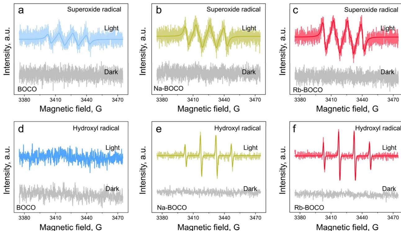
Fig. 3 The EPR-DMPO spectra of  $\cdot\text{O}_2^-$  in samples (a) BOCO, (b) Na-BOCO, and (c) Rb-BOCO under dark conditions and light conditions; the EPR-DMPO spectra of  $\cdot\text{OH}$  in samples (d) BOCO, (e) Na-BOCO, and (f) Rb-BOCO under dark conditions and light conditions.
