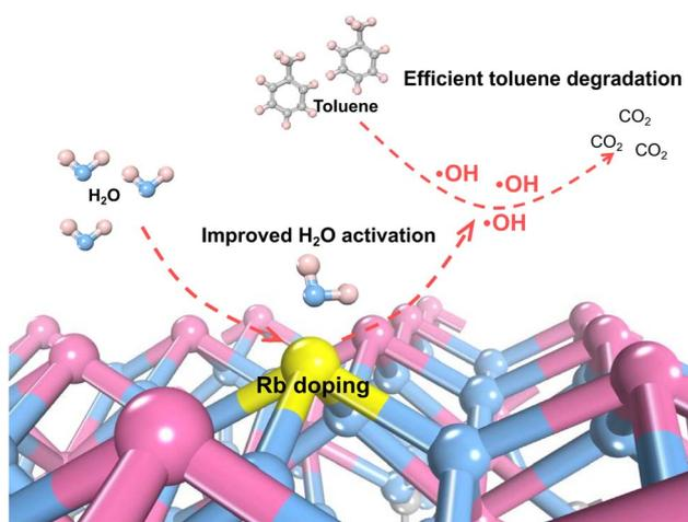
Fig. 6 Schematic diagram illustrating that doping with Rb ions promotes the generation of hydroxyl radicals and enhances the stability of toluene degradation.
