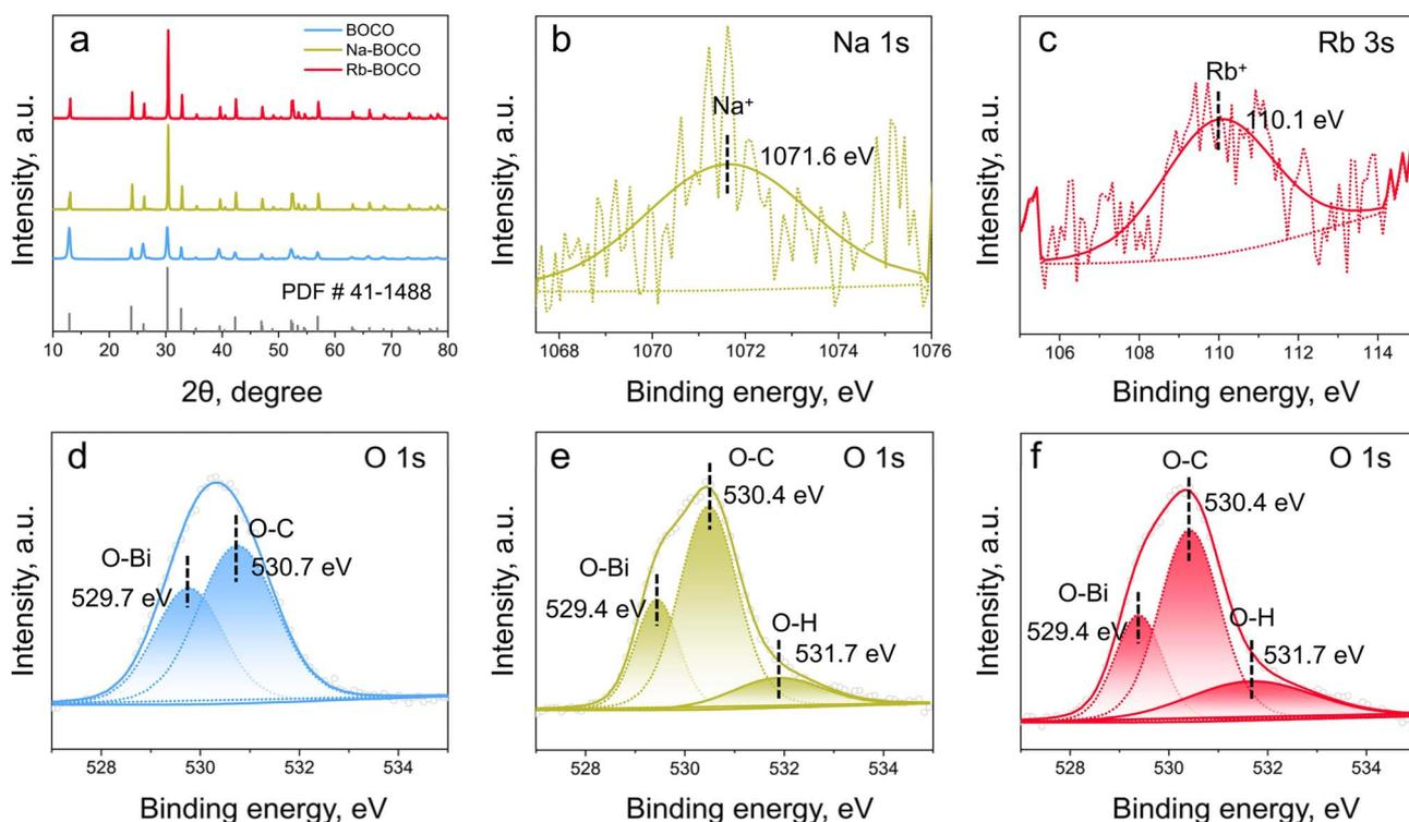
**Fig. 1** (a) XRD pattern of the prepared sample, (b) the high-resolution XPS spectrum (Na 1s) of sample Na-BOCO, (c) the high-resolution XPS spectrum (Rb 3s) of sample Rb-BOCO, and the high-resolution XPS spectrum (O 1s) of (d) BOCO, (e) Na-BOCO, and (f) Rb-BOCO.
