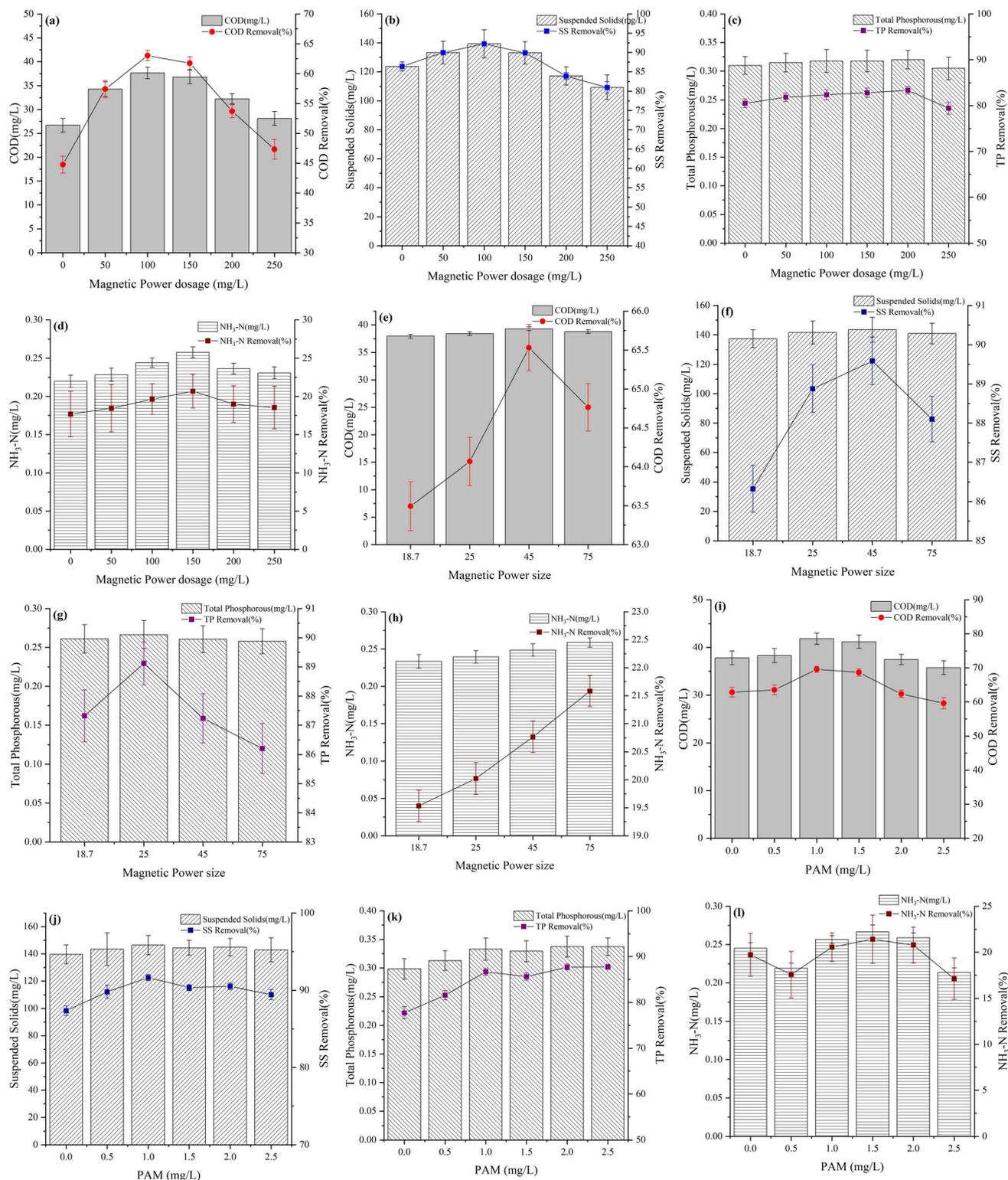
Fig. 1 Removal efficiency of various pollutants by magnetic powder with (a) COD, (b) SS, (c) TP, and (d) NH<sub>3</sub>-N, magnetic particles (different particle sizes): (e) COD, (f) SS, (g) TP, (h) NH<sub>3</sub>-N; and polyacrylamide with (i) COD, (j) SS, (k) TP, and (l) NH<sub>3</sub>-N.
