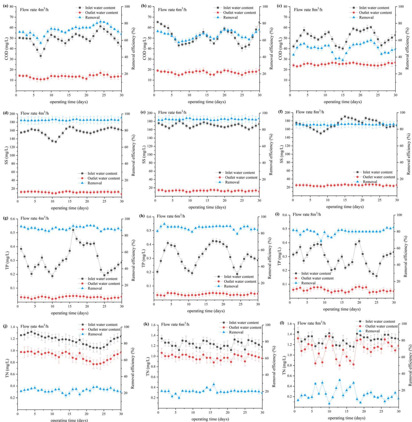
Fig. 7 Removal effect of: (a–c) COD, (d–f) suspended solids, (g–i) total phosphorous, and (j–l) total nitrogen inside the device.
