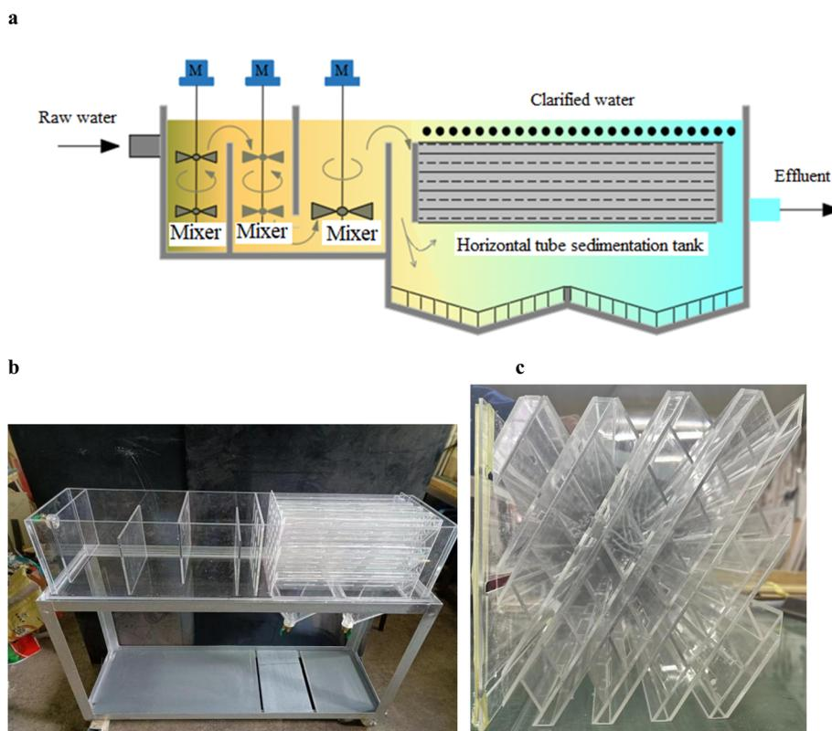
Fig. 6 (a) Schematic of the device; (b) photographic image of the device in the laboratory, and (c) a cross-sectional view of the horizontal tube of the sedimentation separation device.
