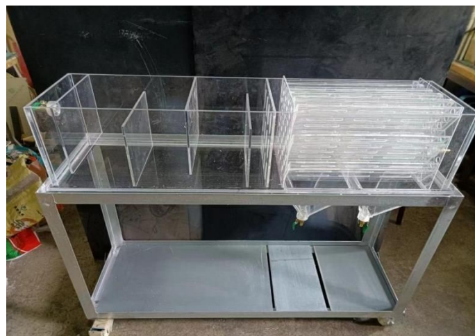
Fig. 6 (a) Schematic diagram of the device, (b) Device photographic image in the laboratory, and (c) Cross-section view of the horizontal tube sedimentation separation device
