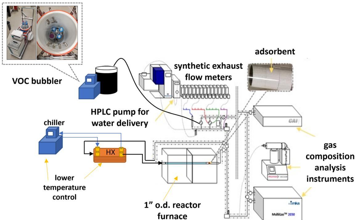
Fig. 2 Schematic of bench reactor layout used for measuring adsorbent's toluene adsorption and desorption behavior from a contaminated air flow.
