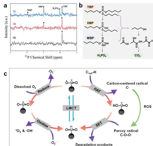
Fig. 5 (a)  $^{31}\text{P}$  NMR spectra acquired at different stages of degradation, (b) schematic diagram of photocatalytic degradation of TBP, and (c) proposed mechanism for the photocatalytic degradation of organic substances by U@GO-1000.
