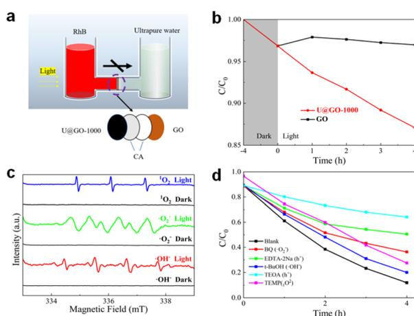
Fig. 4 (a) Schematic diagram of the two-cup experiment. (b) Results of two-cup experiment. (c) ESR spectrum of U@GO-1000; the signals of hydroxyl radicals ( $\cdot\text{OH}$ ), superoxide radicals ( $\cdot\text{O}_2^-$ ) and singlet oxygen ( $^1\text{O}_2$ ) were measured using free radical scavengers respectively in the dark and under light conditions. (d) Results of scavenging experiments.
