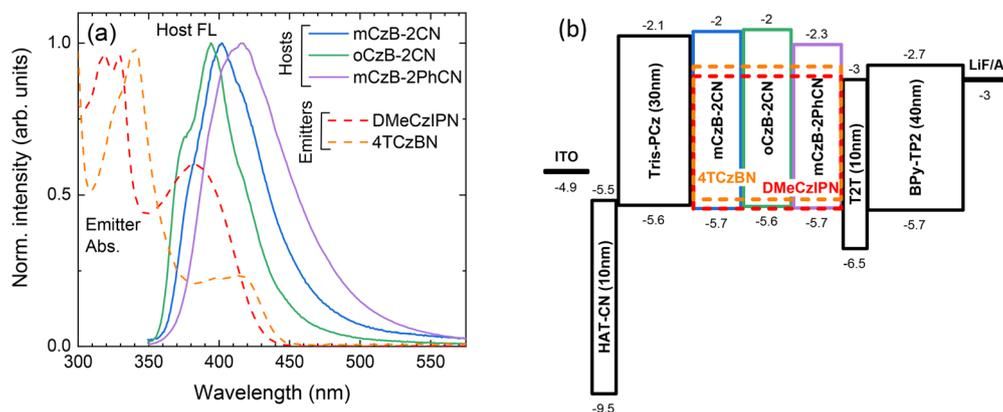
Fig. 6 (a) Absorption spectra of blue TADF emitters (dashed lines) and FL spectra of **mCzB-2CN**, **oCzB-2CN**, and **mCzB-2PhCN** neat films (solid lines). (b) Energy-level diagram of the fabricated TADF-OLEDs using carbazole–biphenyl hosts (**mCzB-2CN**, **oCzB-2CN**, **mCzB-2PhCN**) doped with TADF emitters (4TCzBN and DMeCzIPN). Shown are HOMO/LUMO energies in eV (relative to vacuum) and layer thicknesses in parentheses. Dashed outlines indicate emitter levels within the host layer.
