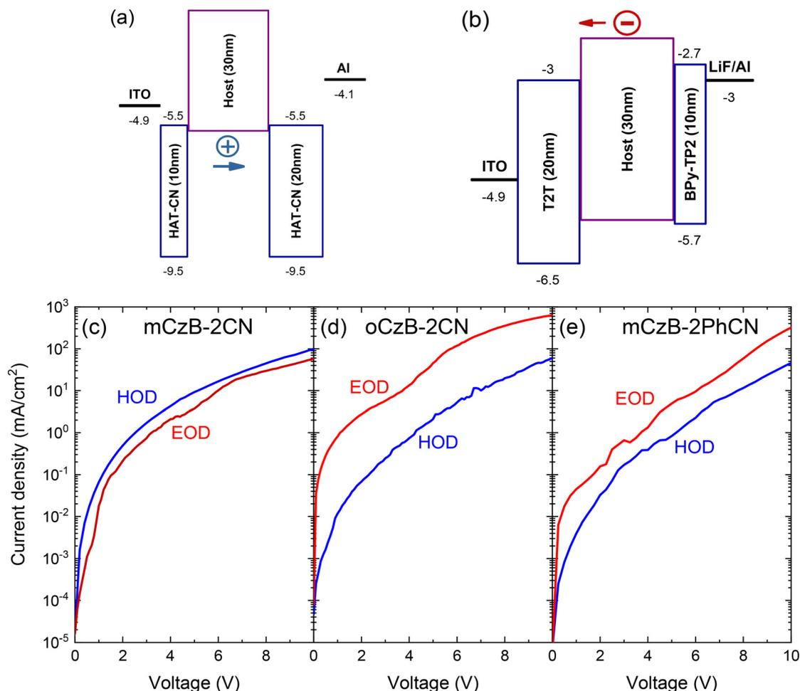
Fig. 5 Single-carrier device characteristics. Energy-level diagrams of (a) hole-only and (b) electron-only devices (energy values in eV), and corresponding current density–voltage ( $J$ – $V$ ) curves of (c) **mCzB-2CN**, (d) **oCzB-2CN**, and (e) **mCzB-2PhCN**. HOD and EOD denote hole-only and electron-only devices, respectively.
