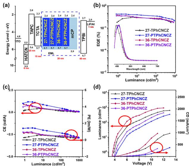
Fig. 7 (a) Energy level diagram of the devices. (b) Normalized EL spectra and EQE versus luminance curves, (c) PE-L-CE curves, and (d)  $J-V-L$  curves of 27-TPhCNCZ, 27-PTPhCNCZ, 36-TPhCNCZ, and 36-PTPhCNCZ in the 10 wt% doped OLED.
