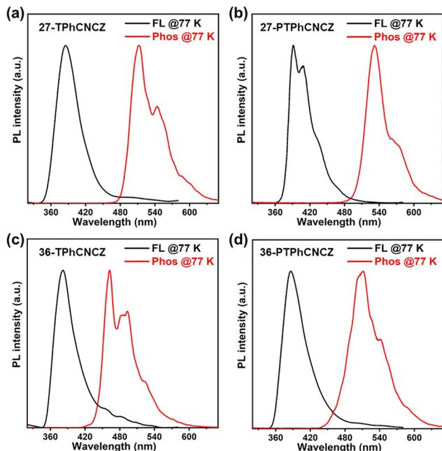
Fig. 6 Phosphorescence measurement diagram and PL spectra of (a) 27-TPhCNCZ, (b) 27-PTPhCNCZ, (c) 36-TPhCNCZ, and (d) 36-PTPhCNCZ in THF (77 K).
