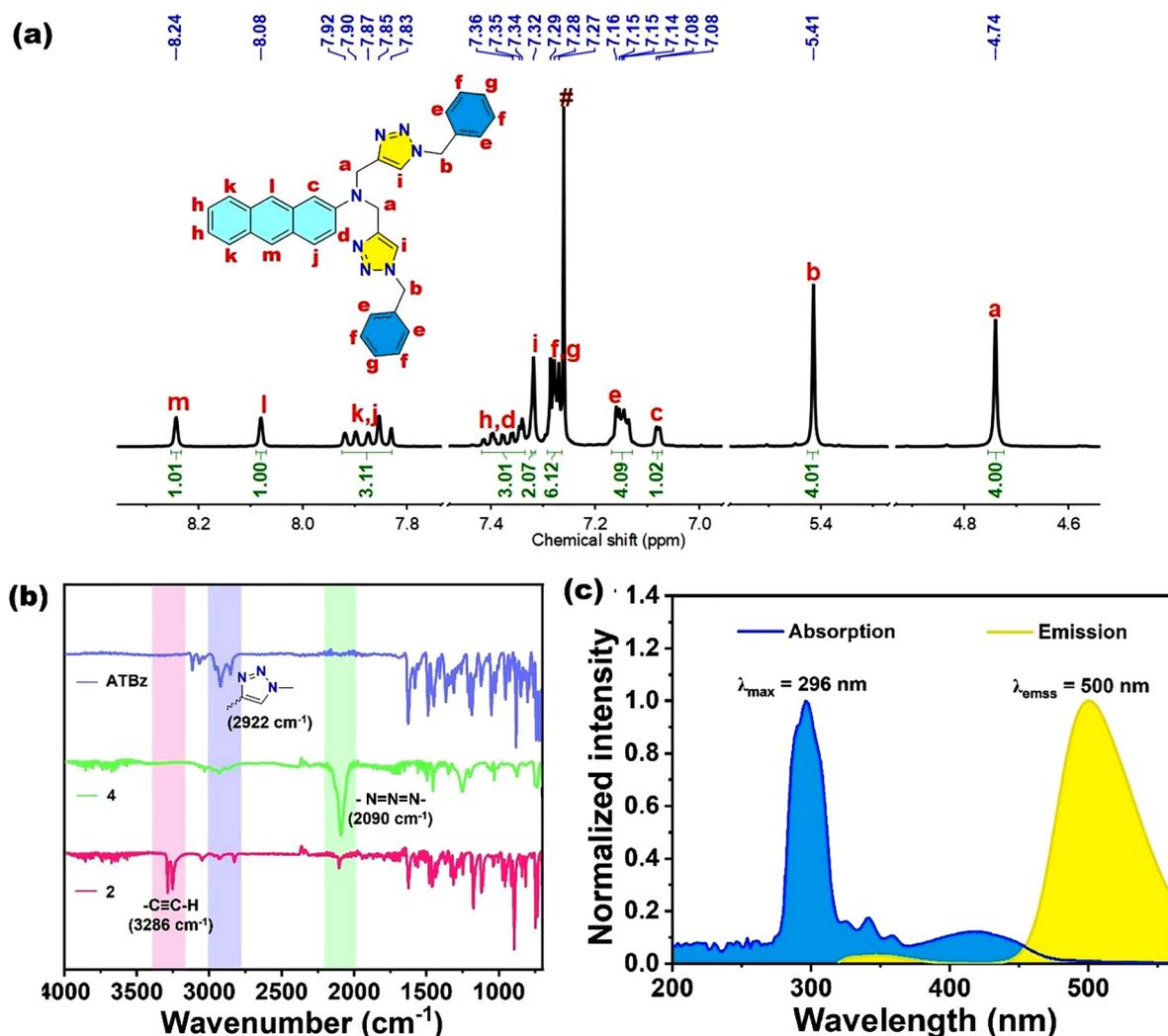
Fig. 1 (a)  $^1\text{H-NMR}$  spectrum of **ATBz** at 400 MHz in  $\text{CDCl}_3$  at 298 K, with (#) denoting the residual proton signal of  $\text{CDCl}_3$ , (b) FT-IR spectrum of **ATBz**, (c) Normalised absorption and emission spectra of **ATBz** (20  $\mu\text{M}$ ) in water (1% DMSO) upon excitation at 296 nm.
