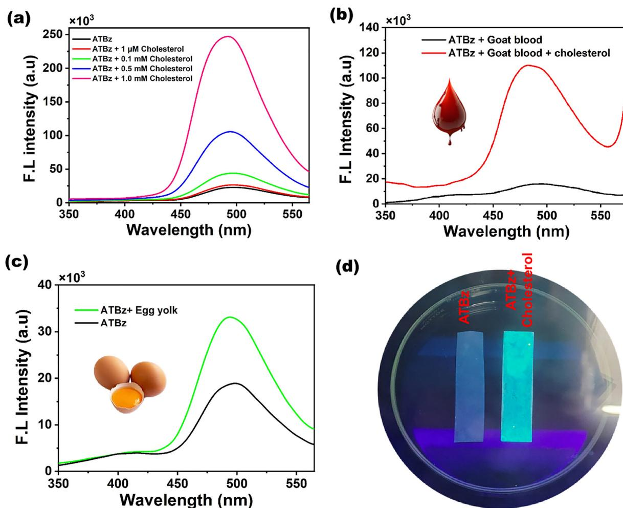
Fig. 4 Detection of cholesterol in (a) human serum, (b) goat blood and (c) egg yolk samples when excited at 296 nm. (d) Photograph of detection of cholesterol using an **ATBz** coated paper-strip under a UV lamp.
