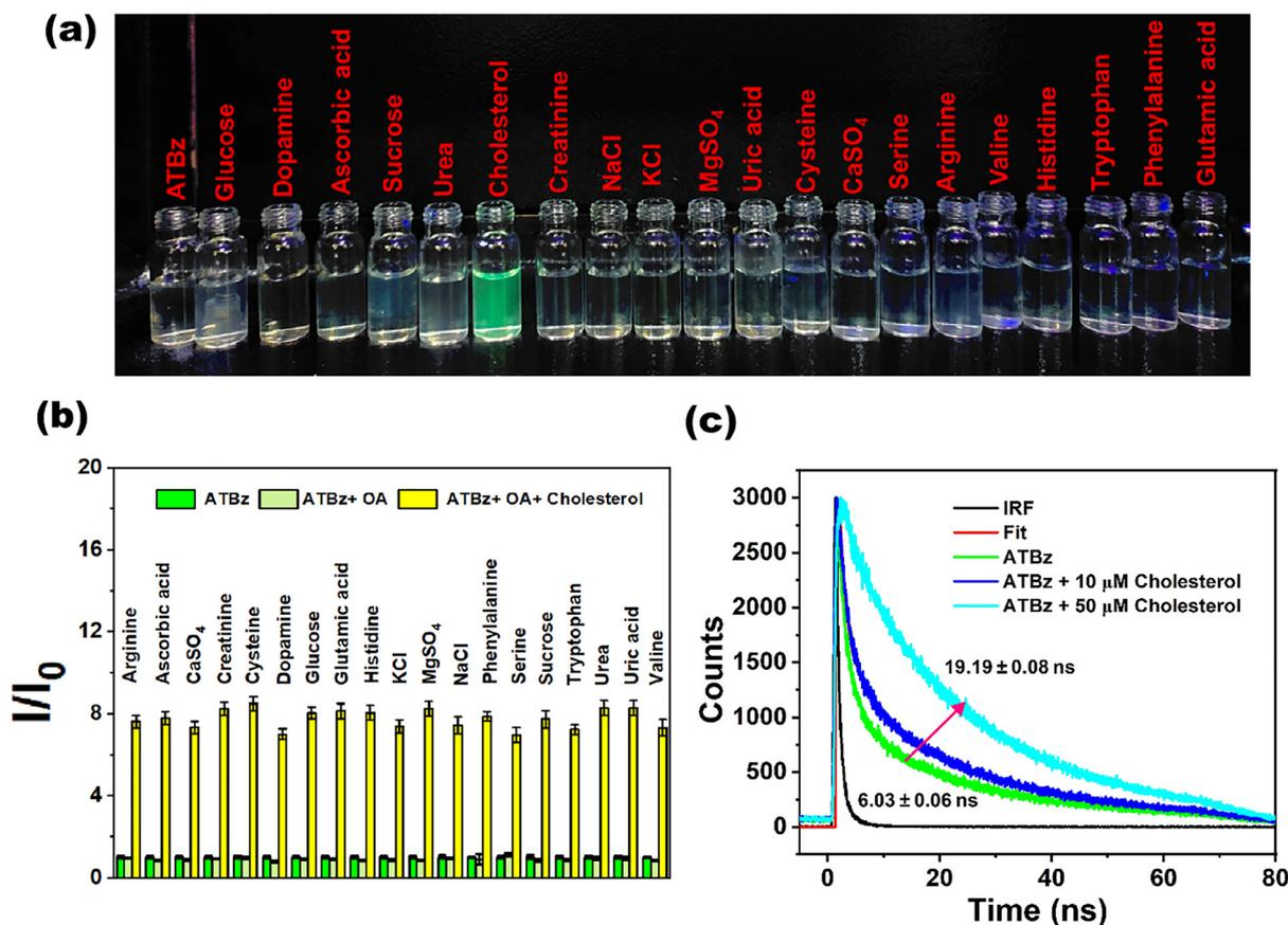
Fig. 3 (a) Photograph of **ATBz** with various analytes (100  $\mu\text{M}$ ) including cholesterol upon illumination under a UV lamp, (b) bar diagram representing competition in the presence of various analytes (OA = other analytes), and (c) the time-resolved fluorescence spectra of **ATBz** with 10 and 50  $\mu\text{M}$  cholesterol concentration.
