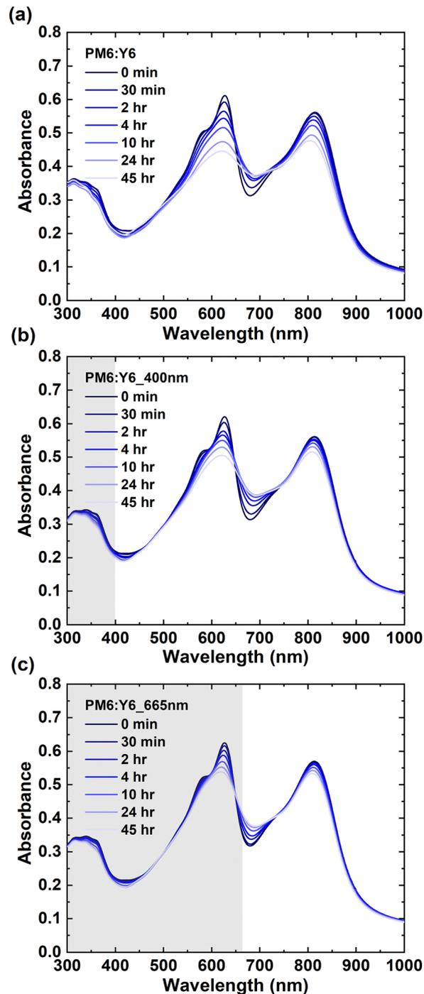
**Fig. 2** The optical absorption spectra of spin-coated PM6:Y6 (1:1) films measured in air before and after photodegradation by exposure for different times (30 min, 2 h, 10 h, 24 h, and 45 h) to AM1.5 light in air without filter (a), with LP400 filter (b), and with LP665 filter (c). The grey area indicates the part of the spectrum that is blocked by the filter during the degradation process.
