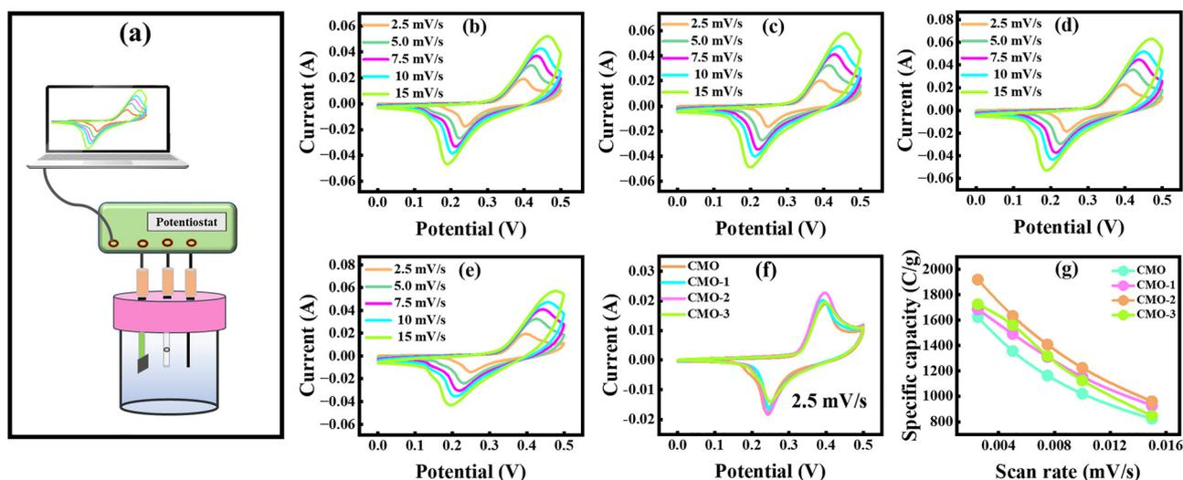
Fig. 3 (a) Schematic of the three-electrode system, (b)–(e) CV profiles of CMO, CMO-1, CMO-2, and CMO-3 at various scan rates, (f) comparative CV curves of all samples at a scan rate of 2.5 mV s<sup>-1</sup>, and (g) variation of specific capacity with scan rate for all the electrodes.
