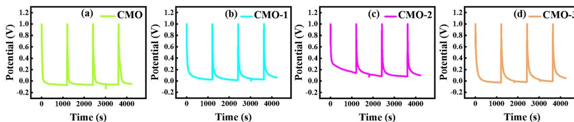
**Fig. 6** (a)–(d) GITT profiles of CMO, CMO-1, CMO-2, and CMO-3, highlighting ion diffusion kinetics at constant current pulses.
