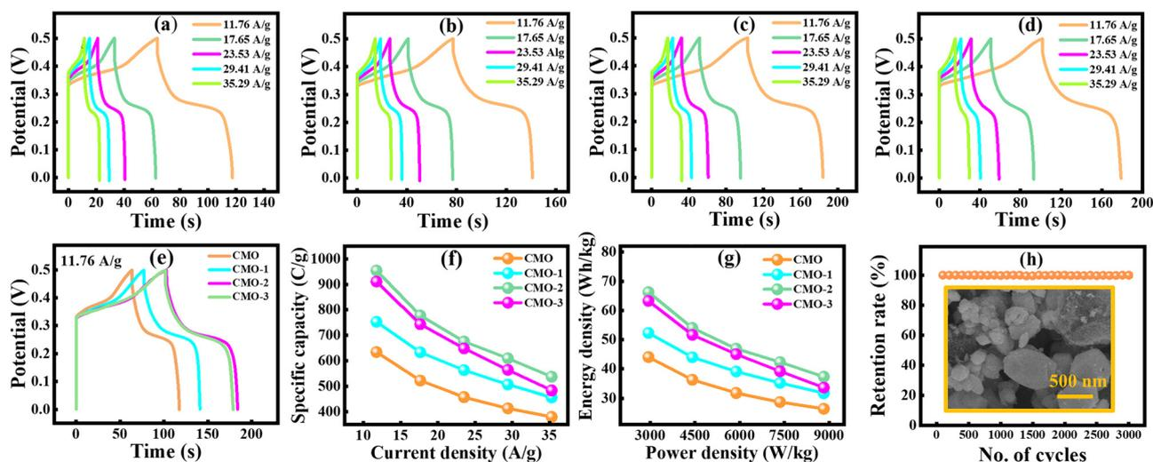
Fig. 5 (a)–(d) GCD profiles of CMO, CMO-1, CMO-2, and CMO-3 at different current densities, (e) comparison of all the electrodes at 11.76 A g<sup>-1</sup>, (f) variation of specific capacity with current density, (g) Ragone plot for all fabricated electrodes, and (h) capacity retention of CMO-2 up to 3000 cycles along with post-cycling FESEM analysis.
