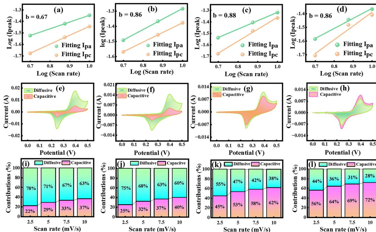
**Fig. 4** (a)–(d) Linear fitting analysis of CMO, CMO-1, CMO-2, and CMO-3 for theoretical evaluation of the charge storage mechanism, (e)–(h) CV plots emphasized the contribution of diffusive and capacitive currents at a scan rate of 2.5 mV s<sup>-1</sup>, and (i)–(l) Dunn model-based analysis of capacitive and diffusive percentage contributions at varying scan rates for all the electrodes.
