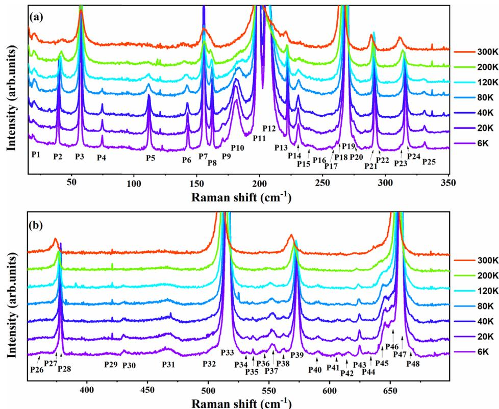
Fig. 1 Temperature evolution of the Raman spectrum in the temperature range of 6 to 300 K, ranging from (a) 15–350  $\text{cm}^{-1}$  and (b) 350–700  $\text{cm}^{-1}$ . The observed phonon modes are labelled as P1–P48.
