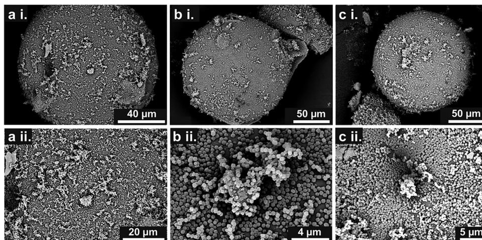
Fig. 2 SEM images of the ZIF-8@SMS\_1hr composite. Three different spheres are shown in images (a) i, (b) i and (c) i. Images (a) ii, (b) ii and (c) ii correspond to the same spheres in (a) and (b) and (c) but at higher magnification.
