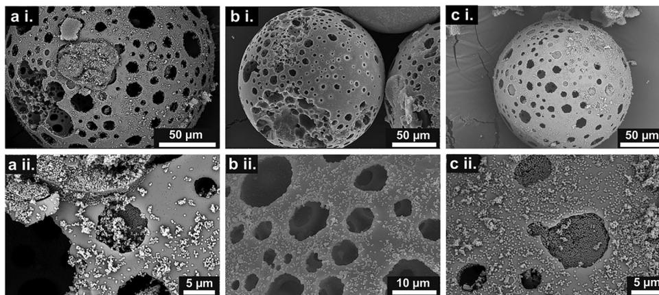
Fig. 3 SEM images of the ZIF-8@PMS\_4.5hr composite showing three different spheres, (a) i (BSE imaging mode), (b) i (SE imaging mode) and (c) i (BSE imaging mode). Images (a) ii, (b) ii and (c) ii correspond to the same spheres but at higher magnification. SE and BSE refer to secondary electron and backscattered electron imaging modes.
