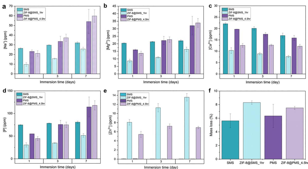
Fig. 5 Ion release profiles and mass loss of the pristine microspheres and composites over a 7-day period, (a)  $[\text{Na}^+]$ , (b)  $[\text{Mg}^{2+}]$ , (c)  $[\text{Ca}^{2+}]$ , (d)  $[\text{P}]$ , (e)  $[\text{Zn}^{2+}]$  and (f) mass loss after 7 days.  $[\text{P}]$  refers to all ionic forms of phosphorus (e.g.  $[\text{PO}_4^{3-}]$ ,  $[\text{HPO}_4^{2-}]$ ,  $[\text{H}_2\text{PO}_4^-]$ ) detected by ICP-MS.
