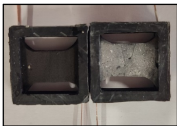
Fig. 1 Left: flat samples of pristine carbon foam with copper contacts inside the plastic casing. Right: the CAU-10-H@CF composite.
