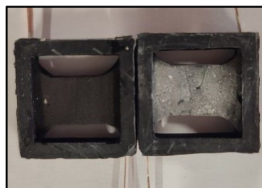
Figure 1: Left: Flat samples of pristine carbon foam with copper contacts inside the plastic casing. Right: The CAU-10-H@CF composite.
