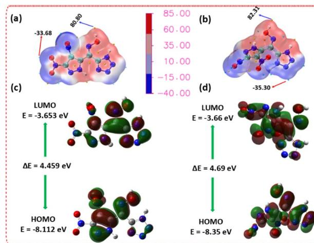
Fig. 5 (a and b) Electrostatic potential (ESP)-mapped van der Waals surfaces of polymorphs **3- $\alpha$**  and **3- $\beta$** , respectively. (c and d) HOMO and LUMO distributions with corresponding HOMO–LUMO energy gaps for **3- $\alpha$**  and **3- $\beta$** .
