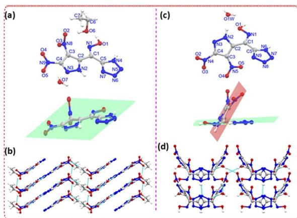
Fig. 2 (a) Asymmetric unit of polymorph **3-α**. (b) Packing arrangement and hydrogen-bonding interactions in **3-α**. (c) Asymmetric unit of polymorph **3-β**. (d) Packing arrangement and hydrogen-bonding interactions in **3-β**.
