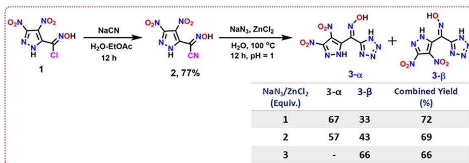
Scheme 1 Synthesis of oxime-bridged pyrazole–tetrazole derivatives 3- $\alpha$  and 3- $\beta$ , showing the effect of NaN<sub>3</sub>/ZnCl<sub>2</sub> equivalents on polymorph distribution and combined yields.
