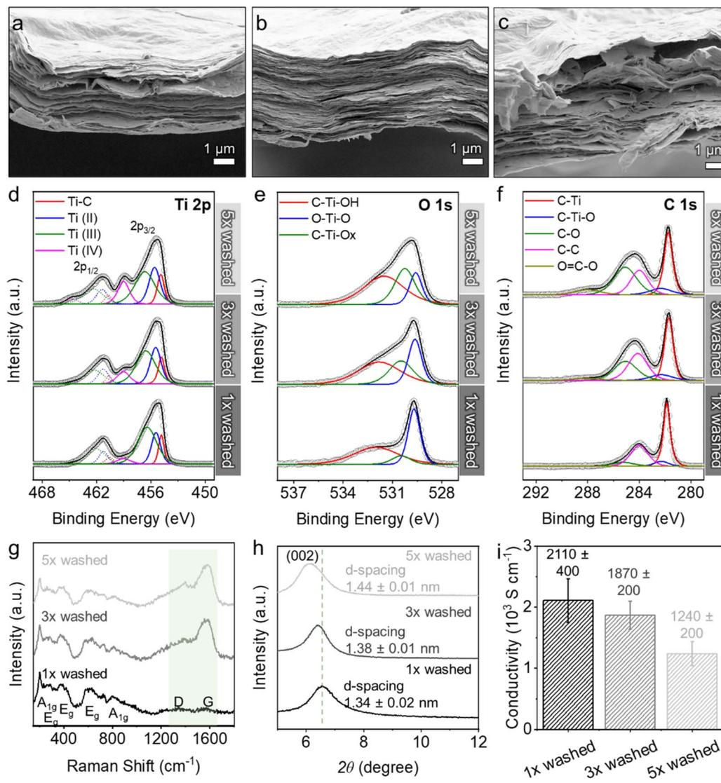
Fig. 2 (a–c) Cross-sectional SEM images of films prepared from 10 mL of 1 mg mL<sup>-1</sup> dispersions of Ti<sub>3</sub>C<sub>2</sub>T<sub>x</sub> MXene sheets washed 1x, 3x, and 5x times in water. (d–f) High-resolution XPS spectra of the films shown in (a–c): stacked (d) Ti 2p, (e) O 1s, and (f) C 1s core-level spectra. (g) Raman spectra, (h) XRD patterns, and (i) electrical conductivity values of the same film samples.
