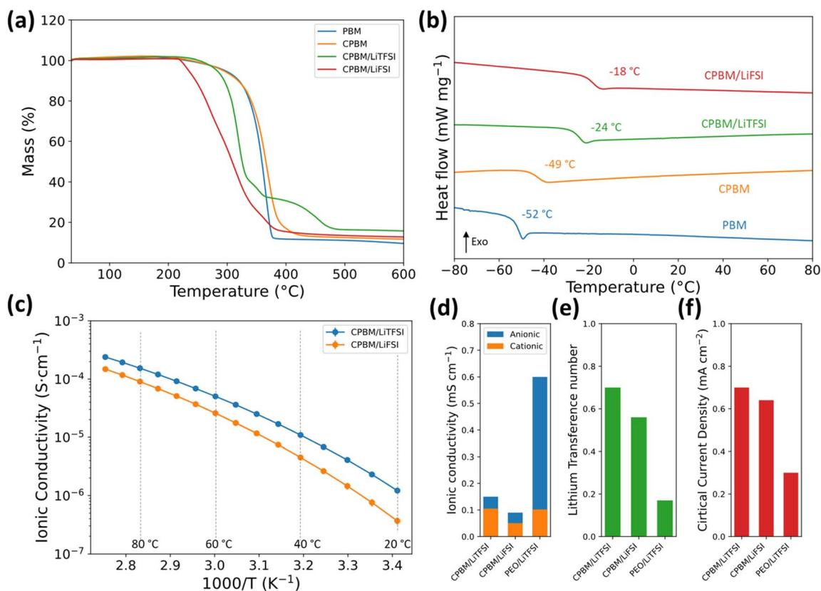
Fig. 2 (a) Thermogram of the PBM polymers and SPEs. (b) DSC traces of the PBM polymers and SPEs. (c) Ionic conductivity of the SPEs as a function of temperature. (d–f) Comparison between CPBM–LiTFSI, CPBM–LiFSI and PEO–LiTFSI SPEs at 80 °C in ionic conductivity, lithium transference number and critical current density, respectively. The data of PEO/LiTFSI were adopted from ref. 46, 48 and 50.
