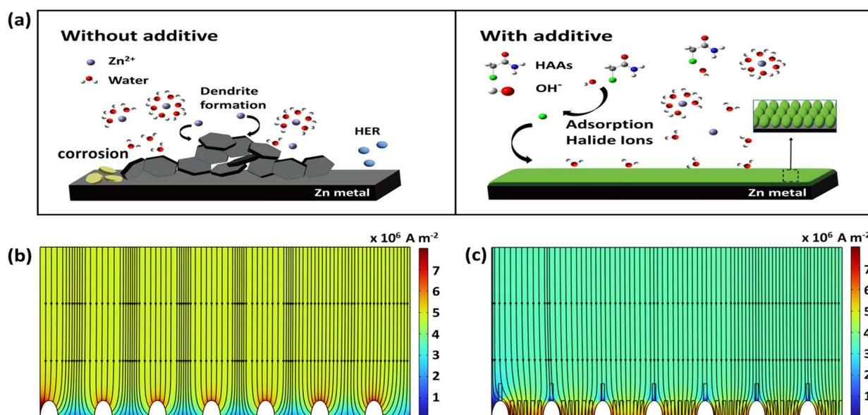
Fig. 2 (a) Schematic illustration showing the protective mechanism of haloacetamide additives. (b and c) COMSOL simulations of Zn<sup>2+</sup> flux distribution in (b) 1 M ZnSO<sub>4</sub> electrolyte and (c) 1 M ZnSO<sub>4</sub> electrolyte containing haloacetamides.
