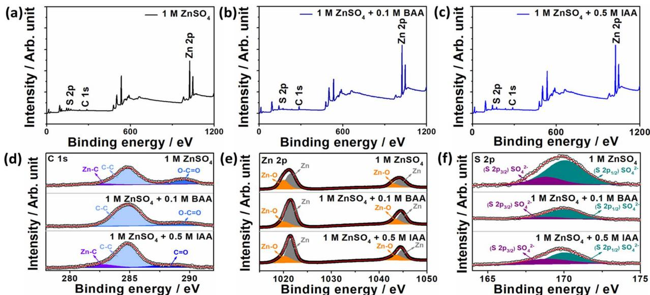
Fig. 5 (a–c) XPS survey spectra of Zn metal electrodes after 10 cycles in (a) 1 M ZnSO<sub>4</sub> electrolyte, (b) 1 M ZnSO<sub>4</sub> electrolyte with bromoacetamide, and (c) 1 M ZnSO<sub>4</sub> electrolyte with iodoacetamide. (d–f) High-resolution (d) C 1s, (e) Zn 2p, and (f) S 2p XPS spectra of Zn metal measured after 10 cycles in 1 M ZnSO<sub>4</sub> electrolytes with and without bromoacetamide or iodoacetamide.
