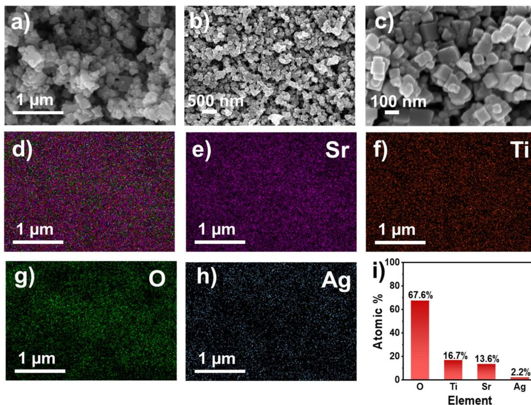
Fig. 2 (a–c) Selected FESEM images of the UL-Ag-STO films. Figures (b) and (c) show the distributed STO crystals within the  $500\ \text{nm}$  and  $100\ \text{nm}$  inset magnifications, respectively. (d–h) EDS elemental mapping highlighting the elemental distributions of STO and underlying Ag in UL-Ag-STO films relative to the FESEM of figure (a). (i) Subsequent atomic ratios tabulated from the EDS spectra.
