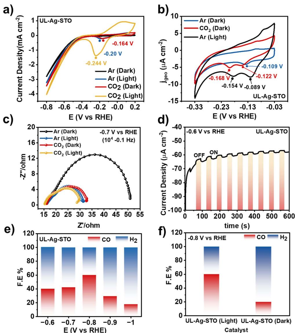
Fig. 3 Photoelectrochemical response of UL-Ag-STO. (a) Cyclic voltammetry (CV) and consequent redox peak under various conditions, (b) zoomed view of Fig. 3(a) showing redox peaks, (c) EIS at  $-0.7 \text{ V vs. RHE}$ , (d) the on-off response, (e) FE under light illumination, and (f) comparison of FE under dark and light conditions.
