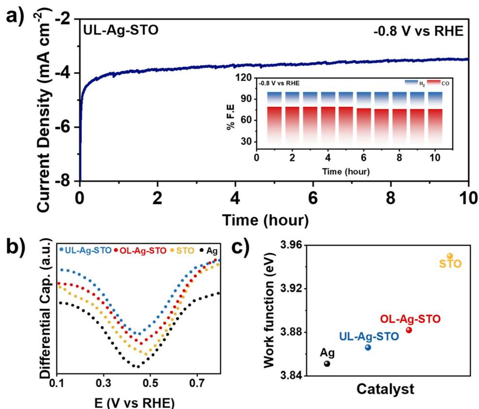
Fig. 5 (a) Long-term stability of CA at  $-0.8$  V vs. RHE for 10 hours with an inset of the photocatalytic performance, (b) differential capacitance measurements, and (c) work function of the various photocathodes estimated from Fig. 5b.
