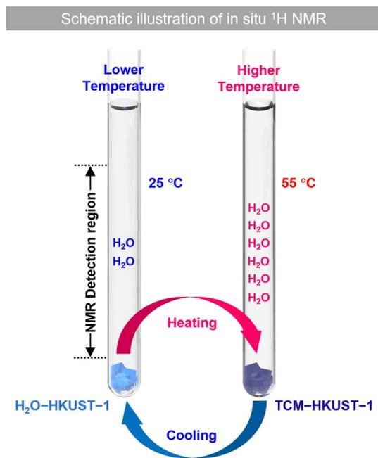
Fig. 6 Schematic illustration of the *in situ*  $^1\text{H}$  NMR setup for probing temperature-dependent coordinative equilibrium: HKUST-1 crystals are immersed in TCM-d containing a defined amount of  $\text{H}_2\text{O}$ , and spectra are recorded at 25 °C and 55 °C during heating/cooling cycles to quantify the fractions of coordinated vs. free  $\text{H}_2\text{O}$  within the NMR detection region. Reproduced with permission from ref. 32, Copyright 2022, Royal Society of Chemistry.
