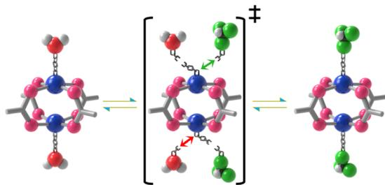
Fig. 3 Schematic illustration of dynamic coordination exchange between  $\text{H}_2\text{O}$  and TCM at a  $\text{Cu}(\text{II})$  paddlewheel OMS; transient  $\text{H}_2\text{O}$  dissociation enables TCM association, establishing a reversible equilibrium (bracketed species denotes the activated encounter complex). Reproduced with permission from ref. 32, Copyright 2022, Royal Society of Chemistry.
