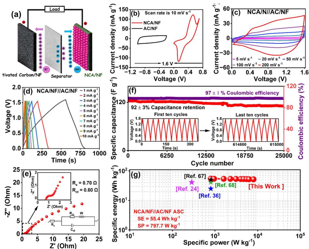
Fig. 4 (a) Illustration of asymmetric supercapacitor (b) the voltage window of AC/NF and NCA/NF at  $10 \text{ mV s}^{-1}$  (c) CV curves at various scan rates ( $5\text{--}200 \text{ mV s}^{-1}$ ), (d) GCD curves at various current densities ( $1\text{ to }10 \text{ mA g}^{-1}$ ), (e) Nyquist plot, (f) cycling stability; standard deviations are shown to indicate electrode to electrode variability in cyclic stability and coulombic efficiency, (g) Ragone plot of NCA/NF//AC/NF ASC device.
