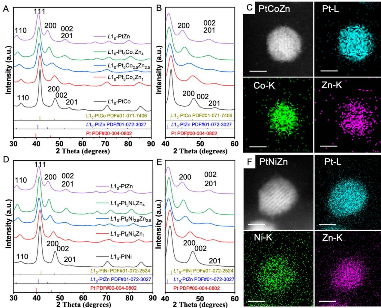
Fig. 3 Characterization of  $L_{10}$ -Pt(M,Zn)/C NPs. (A and B) XRD patterns of  $L_{10}$ -Pt(Co,Zn)/C. (C) STEM image and corresponding elemental mapping images of a single  $L_{10}$ -Pt<sub>5</sub>Co<sub>4</sub>Zn<sub>2.5</sub> NP. (D and E) XRD patterns of  $L_{10}$ -Pt(Ni,Zn)/C NPs. (F) STEM image and corresponding elemental mapping images of a single  $L_{10}$ -Pt<sub>5</sub>Ni<sub>2.5</sub>Zn<sub>2.5</sub> NP (Pt: blue, Co or Ni: green, Zn: purple).
