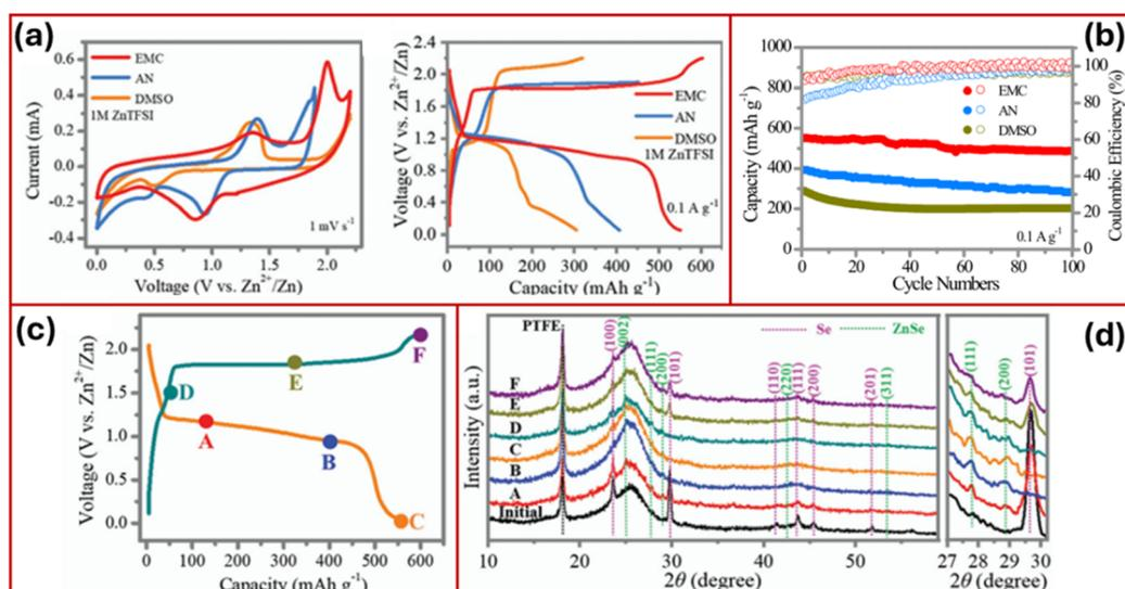
Fig. 3 Electrochemical performance of the Zn–Se battery with organic electrolytes. (a) CV curves at  $1 \text{ mV s}^{-1}$  and (b) GCD curves at  $0.1 \text{ A g}^{-1}$  based on 1 M ZnTFSI in EMC, AN, and DMSO at  $1 \text{ mV s}^{-1}$ , respectively. (c) GCD profile and (d) *ex situ* XRD patterns at selected potentials.<sup>51</sup> Reproduced from ref. 51 with permission from Royal Society of Chemistry, copyright, 2019.
