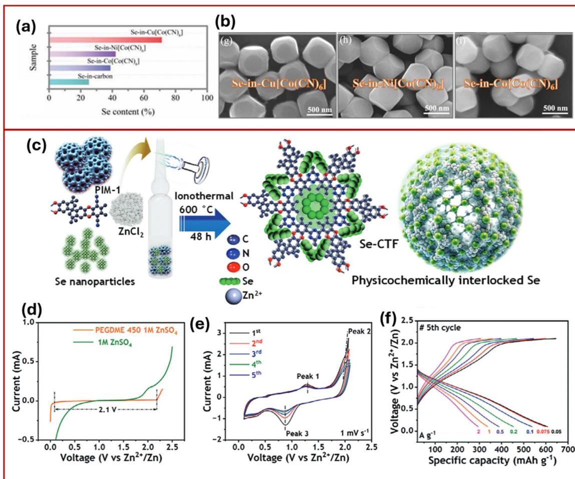
Fig. 7 (a) The Se content in porous carbon and (b) SEM images of PBA frameworks.<sup>66</sup> Reproduced from ref. 66 with permission from Wiley-VCH, copyright 2022. (c) Schematic depiction of Se-CTF cathode preparation, (d) LSV curves of 1 M ZnSO<sub>4</sub> in PEGDME 450, (e) CV curve of Se-CTF cathode at 1 mV s<sup>-1</sup>, and (f) CD profile at different current rates.<sup>67</sup> Reproduced from ref. 67 with permission from Wiley-VCH, copyright 2024.
