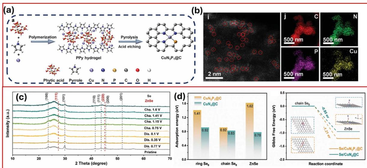
Fig. 6 (a) Synthesis process of and (b) enlarged EDS elemental mapping of CuN<sub>3</sub>P<sub>1</sub>@C, (c) *ex situ* XRD patterns, (d) adsorption energy of CuN<sub>3</sub>P<sub>1</sub>@C and CuN<sub>4</sub>@C to ring Se<sub>8</sub>, chain Se<sub>8</sub>, and ZnSe, and Gibbs free energy.<sup>64</sup> Reproduced from ref. 64 with permission from Wiley-VCH, copyright 2025.
