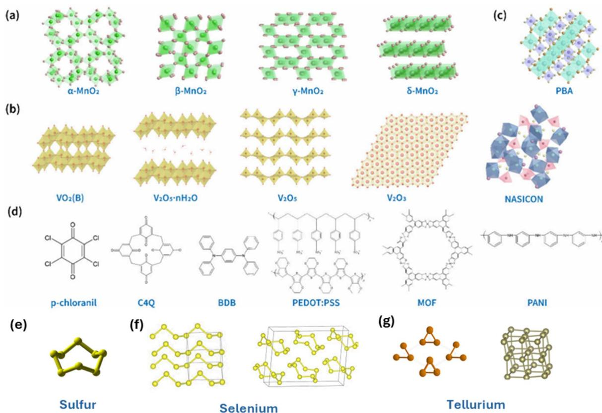
Fig. 2 Structures of various cathode materials for AZIBs: (a) manganese oxides, (b) vanadium oxides and vanadates, (c) Prussian blue analogues, (d) organic and metal–organic frameworks.<sup>29</sup> Reproduced from ref. 29 with permission from American Chemical Society, copyright 2025. Structures of (e) sulfur, (f) selenium, and (g) tellurium.
