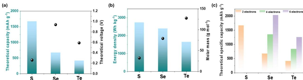
Fig. 1 Physicochemical properties of chalcogens (S, Se, and Te): (a) theoretical capacity, (b) energy density, and (c) theoretical specific capacity.<sup>16</sup>
