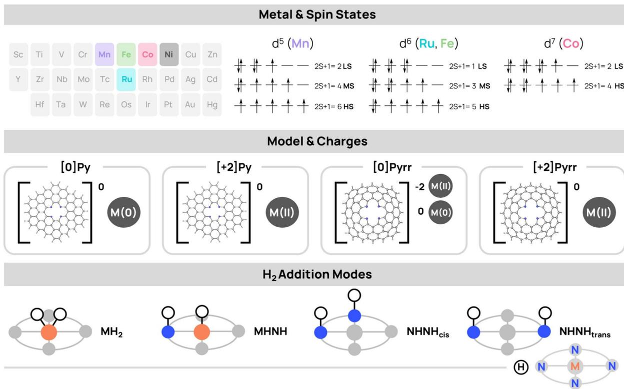
Fig. 2 Metals (Mn, Ru, Fe, Co), spin states (singlet, doublet, triplet, quartet, quintet, sextet), models (pyridinic: Py, and pyrrolic: Pyrr), charges ([0] or [+2]) for the studied model of N-doped graphene-based SACs, and the H<sub>2</sub> addition modes considered (MH<sub>2</sub>, MHNH, NHNH<sub>trans</sub>, NHNH<sub>cis</sub>). For the H<sub>2</sub> addition modes, spheres in orange, blue, white, and grey represent metal, nitrogen, hydrogen, and carbon atoms, respectively.
