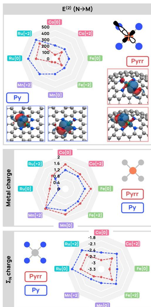
Fig. 5 Stabilization energies ( $E^{(2)}$ ) from nitrogen-to-metal orbital donor-acceptor interaction (top), natural charges of the metal center (middle), and total nitrogen natural charges ( $\sum N$ , bottom) across all metal and charge states. Blue points represent Py systems, red points represent Pyrr systems.
