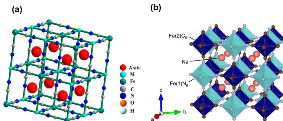
Fig. 8 Schematic illustration of a general (a) Prussian blue analogue (PBA), reproduced from ref. 81 with permission from American Chemical Society, copyright 2023 and (b) of  $\text{Na}_{2-x}\text{FeFe}(\text{CN})_6$ , reproduced from ref. 80 with permission from Springer Nature, copyright 2020.
