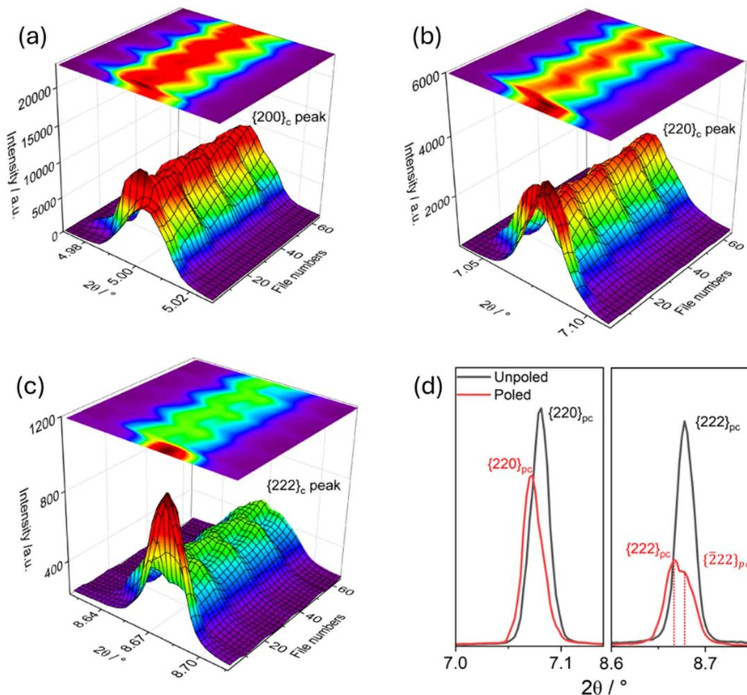
Fig. 8 3D and contour maps of (a)  $\{200\}_c$  (b)  $\{220\}_c$  and (c)  $\{222\}_c$  XRD profiles at  $\psi = 0^\circ$  of the  $x = 0.44$  ceramic during *in situ* poling synchrotron XRD. (d) Synchrotron XRD profiles at  $\psi = 0^\circ$  of unpoled (virgin) and poled specimens of the  $x = 0.44$  ceramic.
