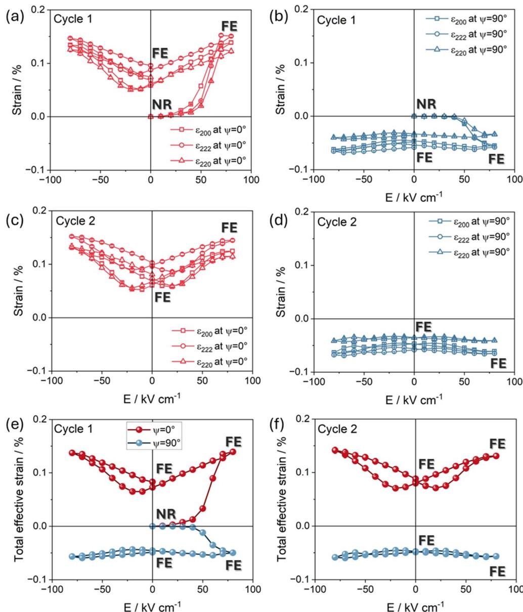
Fig. 9 Effective strain at (a)  $\psi = 0^\circ$  and (b)  $\psi = 90^\circ$  during the first cycle of electric field. Effective strain at (c)  $\psi = 0^\circ$  and (d)  $\psi = 90^\circ$  during the second cycle of electric field. Total effective strain during the (e) first cycle and (f) second cycle of electric field.
