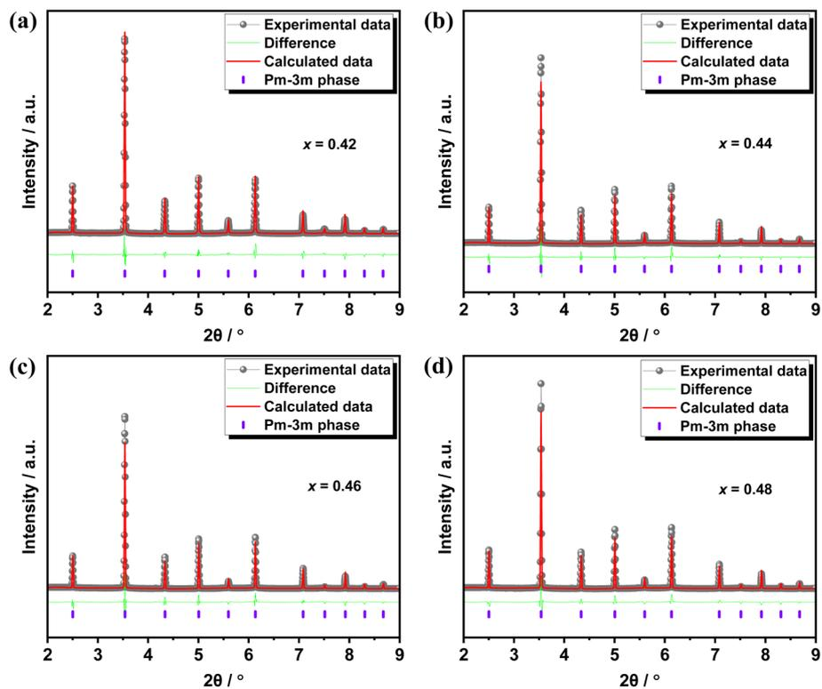
Fig. 2 Room temperature synchrotron XRD pattern and corresponding Rietveld refinement results for  $(1-x)\text{BF}-x\text{ST}$  ceramics, (a)  $x = 0.42$ , (b)  $x = 0.44$ , (c)  $x = 0.46$ , and (d)  $x = 0.48$ .
