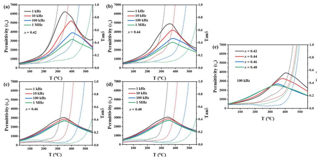
Fig. 5 (a) The temperature dependence of dielectric permittivity ( $\epsilon_r$  vs.  $T$ ) and loss ( $\tan \delta$  vs.  $T$ ) of  $(1-x)\text{BF}-x\text{ST}$  ceramics, (a)  $x = 0.42$ , (b)  $x = 0.44$ , (c)  $x = 0.46$ , (d)  $x = 0.48$ , and (e) The temperature dependence of  $\epsilon_r$  and  $\tan \delta$  compared at 100 kHz.
