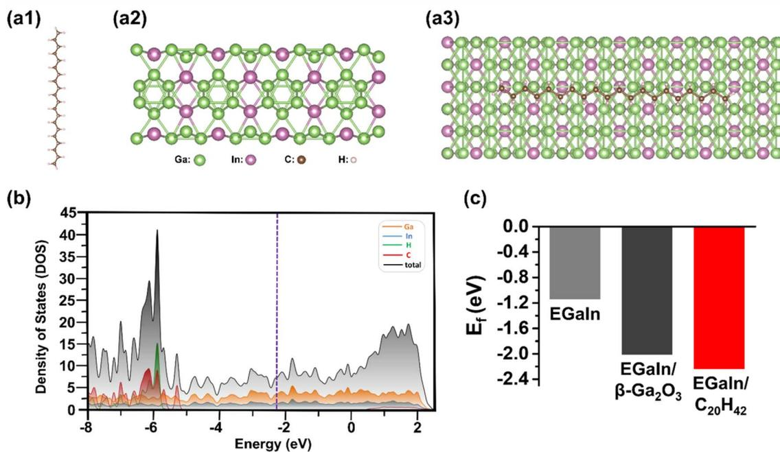
Fig. 6 DFT optimized geometries of (a1)  $C_{20}H_{42}$  and (a2) the (100) hexagonal EGaIn surface, and (a3)  $C_{20}H_{42}$ -adsorbed EGaIn surface at its most favorable configuration. (b) Density of states (DOS) of the EGaIn- $C_{20}H_{42}$  hybrid, where the dotted vertical line (purple color) represents the Fermi energy level ( $E_f = -2.24$  eV). (c) Calculated  $E_f$  values for different interfacial compositions.
