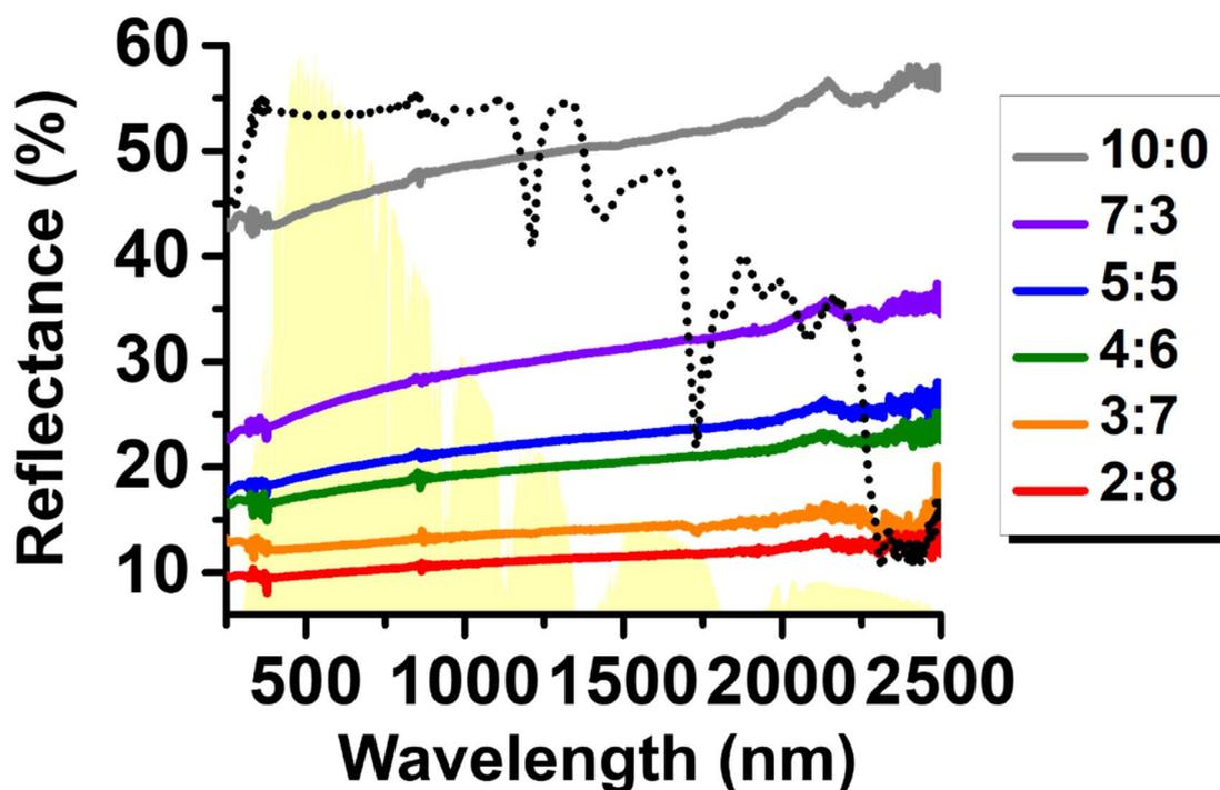
Fig. 9 Relative reflectance of broadband light (250–2500 nm) by the hybrid-coated surfaces with various EGaIn : C<sub>20</sub>H<sub>42</sub> volume ratios. The dotted black line corresponds to the surface coated with C<sub>20</sub>H<sub>42</sub>-only (0 : 10) particles. The yellow shading represents the AM 1.5G solar spectrum.
