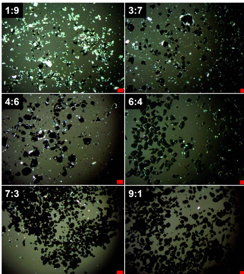
Fig. 2 Polarized light microscopy images of the EGaIn–C<sub>20</sub>H<sub>42</sub> hybrid particles at selected EGaIn : C<sub>20</sub>H<sub>42</sub> volume ratios (scale bars: 100 μm).
