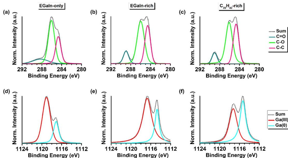
Fig. 7 XPS (a-c) C 1s and (d-f) Ga 2p narrow scan spectra for the surfaces coated with pure EGaIn (EGaIn :  $C_{20}H_{42}$  = 10 : 0; a and d), EGaIn-rich hybrid (EGaIn :  $C_{20}H_{42}$  = 7 : 3; b and e), and  $C_{20}H_{42}$ -rich hybrid (EGaIn :  $C_{20}H_{42}$  = 3 : 7; c and f) particles.
