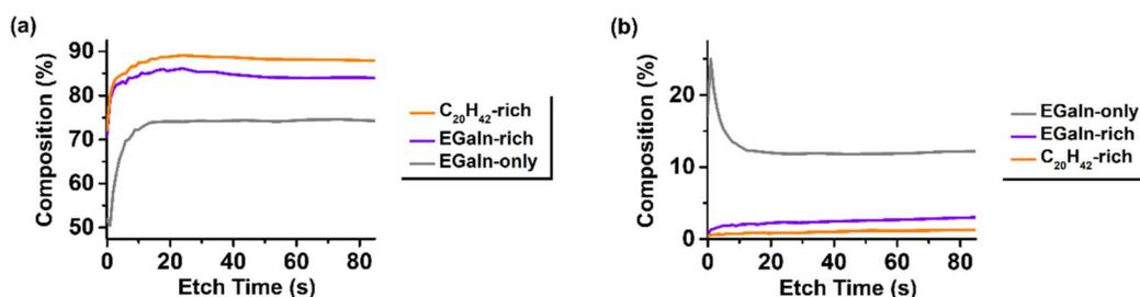
Fig. 8 Depth profiling analysis of the surfaces coated with pure EGaIn (EGaIn : C<sub>20</sub>H<sub>42</sub> = 10 : 0), EGaIn-rich hybrid (EGaIn : C<sub>20</sub>H<sub>42</sub> = 7 : 3), and C<sub>20</sub>H<sub>42</sub>-rich hybrid (EGaIn : C<sub>20</sub>H<sub>42</sub> = 3 : 7) particles. Atomic compositions (%) of (a) C and (b) Ga elements are shown as functions of etch time.
