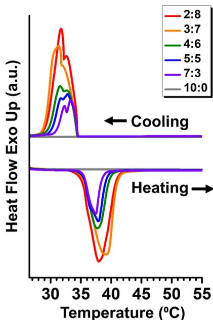
Fig. 4 DSC heating and cooling curves of the EGaIn–C<sub>20</sub>H<sub>42</sub> hybrid particles at selected EGaIn : C<sub>20</sub>H<sub>42</sub> volume ratios. Baseline corrections were applied to all overlapping data, and normalization was performed with respect to the maximum heat flow peak.
