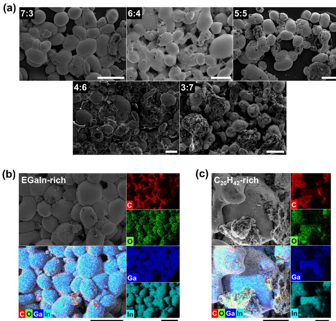
Fig. 3 (a) SEM images of the EGaIn–C<sub>20</sub>H<sub>42</sub> hybrid particles at selected EGaIn : C<sub>20</sub>H<sub>42</sub> volume ratios (scale bars: 100 μm). SEM/EDS analysis of the hybrid particles with (b) EGaIn-rich (7 : 3) and (c) C<sub>20</sub>H<sub>42</sub>-rich (3 : 7) compositions (scale bars in b: 100 μm; scale bars in c: 50 μm).
