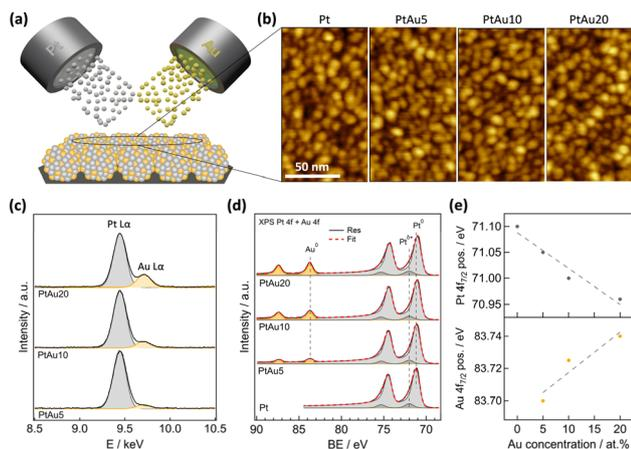
**Fig. 1** (a) Illustration of the magnetron sputtering deposition process, (b) AFM images of the as-deposited pure Pt and Pt–Au alloy catalysts, (c) EDX and (b) XPS spectra acquired for the as-deposited Pt–Au alloy catalysts and pure Pt, and (e) Pt 4f<sub>7/2</sub> and Au 4f<sub>7/2</sub> peak positions extracted from the XPS spectra shown in (d).
