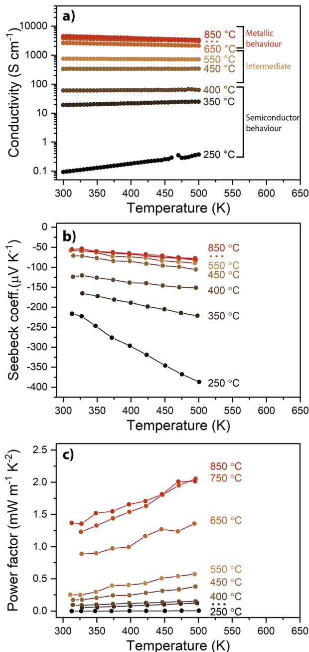
Fig. 5 Temperature-dependent electrical and thermoelectric characteristics of the films deposited at different deposition temperatures on *c*-sapphire: (a) electrical conductivity, (b) Seebeck coefficient and (c) TE power factor.
