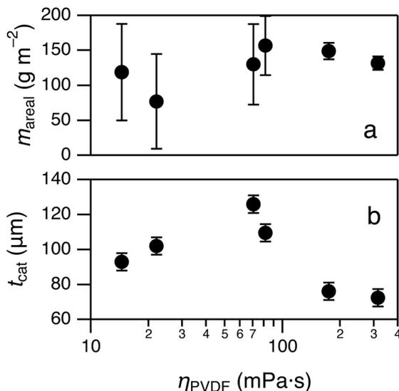
Fig. 8 Properties of formed cathodes of NMC811/CB/PVDF (95 : 5 : 5 w/w/w) across a series of different PVDF/NMP solution viscosities,  $\eta_{\text{PVDF}}$ . (a) Areal mass loading,  $m_{\text{areal}}$ , of the composite cathodes and (b) thicknesses of cathodes produced using a draw down velocity of  $5.8 \text{ mm s}^{-1}$  and a gap height of  $285 \mu\text{m}$  (see SI Table 8 for full characterisation of these cathodes.).
