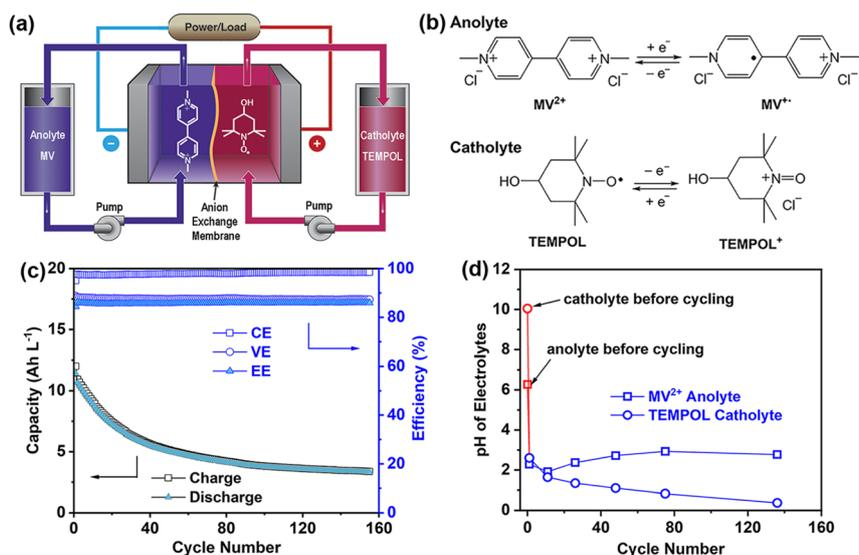
Fig. 1 The  $TEMPOL/MV^{2+}$  RFB system: (a) a schematic illustration; (b) electrochemical reactions of both redoxmers; (c) cycling efficiencies and capacities with 0.5 M redoxmers at  $10 \text{ mA cm}^{-2}$ ; (d) pH values of the anolyte and catholyte over the cycling in Panel (c).
