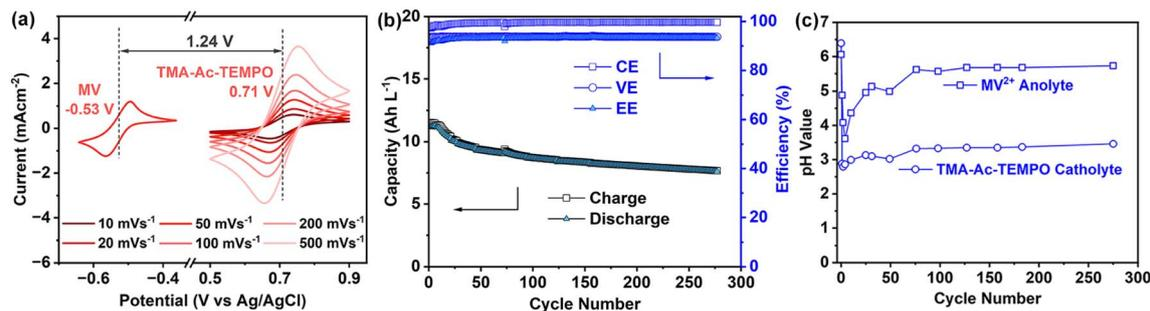
Fig. 6 Stability testing for TMA-Ac-TEMPO: (a) CV scans of 10 mM TMA-Ac-TEMPO and 10 mM  $MV^{2+}$ , respectively, both in 0.5 M NaCl; (b) cycling efficiencies and capacities of a 0.5 M TMA-Ac-TEMPO/ $MV^{2+}$  flow cell at  $10 \text{ mA}\cdot\text{cm}^{-2}$ ; (c) pH values of the anolyte and catholyte over the cycling in panel (b).
