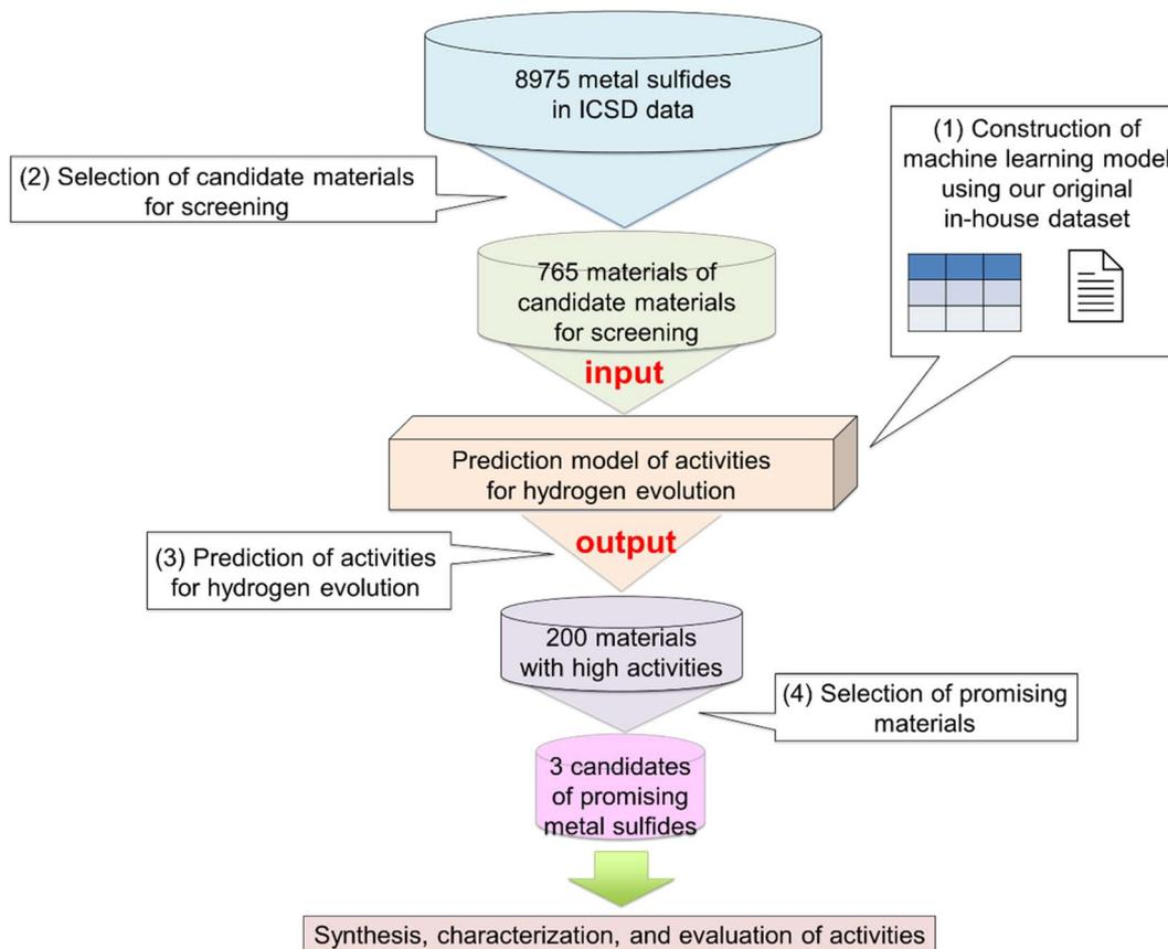
Fig. 1 Flowchart of exploring metal sulfides for H<sub>2</sub> evolution by machine-learning.
