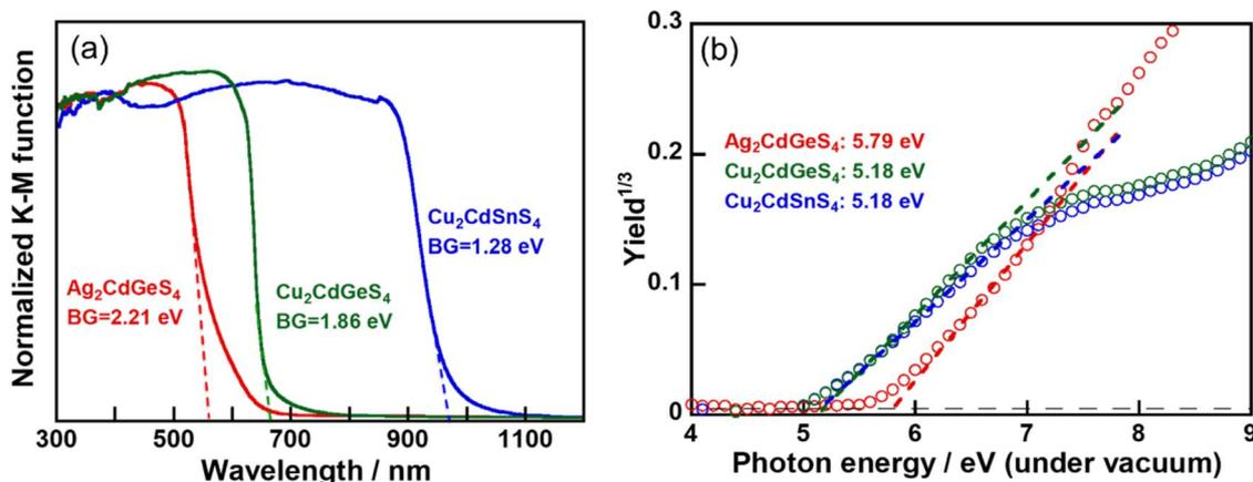
Fig. 5 (a) Diffuse reflectance spectra and (b) PYS spectra of Ag<sub>2</sub>CdGeS<sub>4</sub> and Cu<sub>2</sub>CdMS<sub>4</sub> (M = Ge and Sn) prepared by a solid-state reaction.
