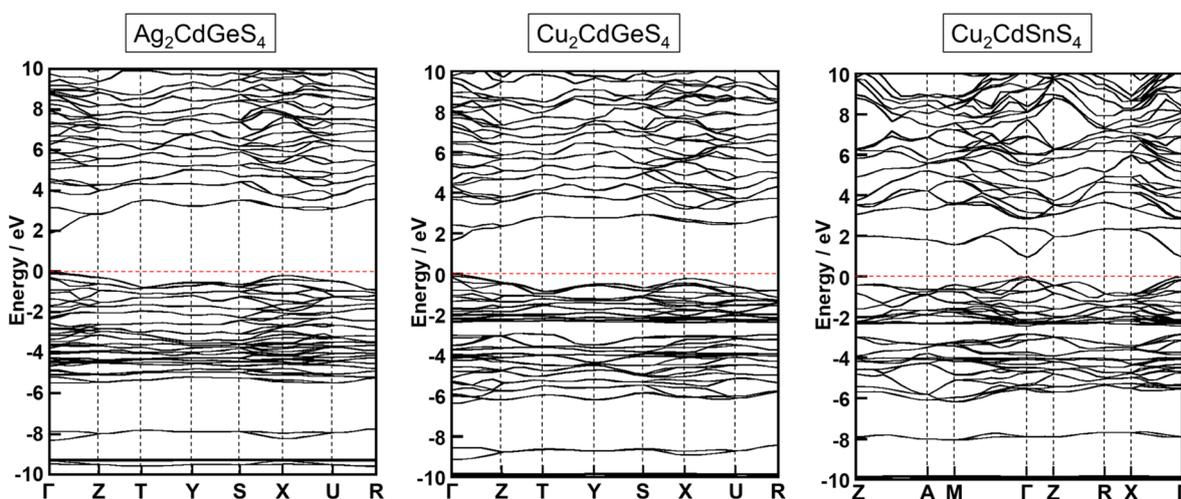
Fig. 6 Band structures of Ag<sub>2</sub>CdGeS<sub>4</sub> and Cu<sub>2</sub>CdMS<sub>4</sub> (M = Ge and Sn).
