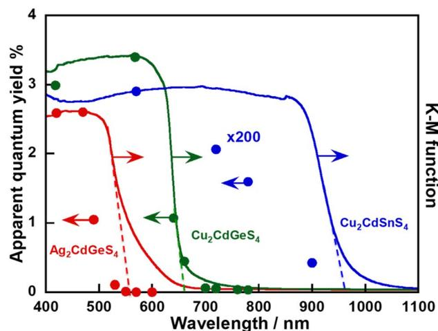
Fig. 10 Action spectra of sacrificial  $\text{H}_2$  evolution over the Ru (0.5 wt%)-loaded  $\text{Ag}_2\text{CdGeS}_4$ ,  $\text{Cu}_2\text{CdMS}_4$  ( $M = \text{Ge}$  and  $\text{Sn}$ ) photocatalysts. Photocatalyst: 0.3 g, cocatalyst: PD *in situ*, reactant solution: 0.5 mol per L  $\text{K}_2\text{SO}_3$  and 0.1 mol per L  $\text{Na}_2\text{S}$  aqueous solution (120 mL), cell: top-irradiation cell with a Pyrex window, light source: 300 W Xe lamp with band-pass filters.
