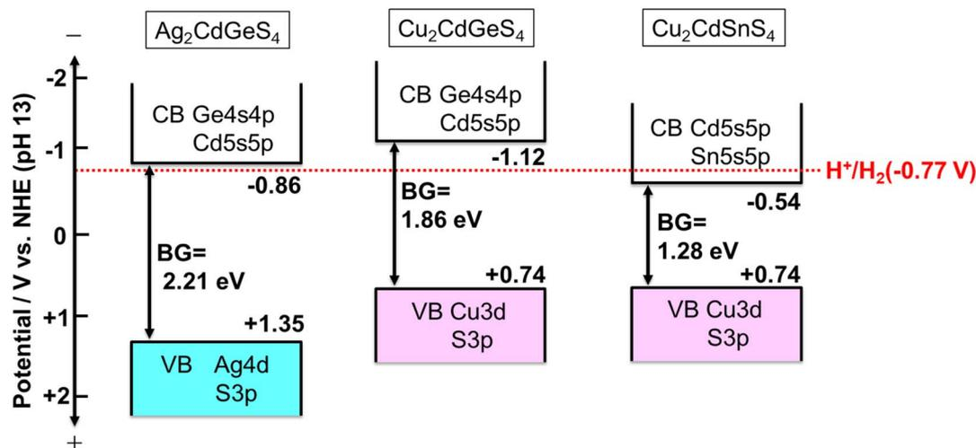
Fig. 8 Band structures of  $\text{Ag}_2\text{CdGeS}_4$  and  $\text{Cu}_2\text{CdMS}_4$  ( $M = \text{Ge}$  and  $\text{Sn}$ ).
