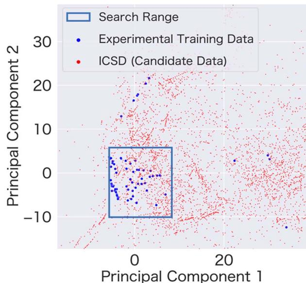
Fig. 3 Material space of metal sulfides in the ICSD and our original dataset by PCA. Principal components 1 and 2 (with no units), which form the axes, are new coordinate axes constructed by performing linear combinations of the original variables.
