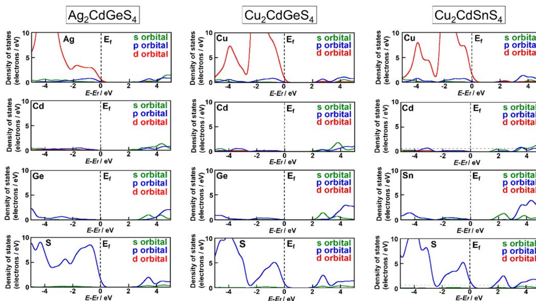
Fig. 7 Density of states of Ag<sub>2</sub>CdGeS<sub>4</sub> and Cu<sub>2</sub>CdMS<sub>4</sub> (M = Ge and Sn).
