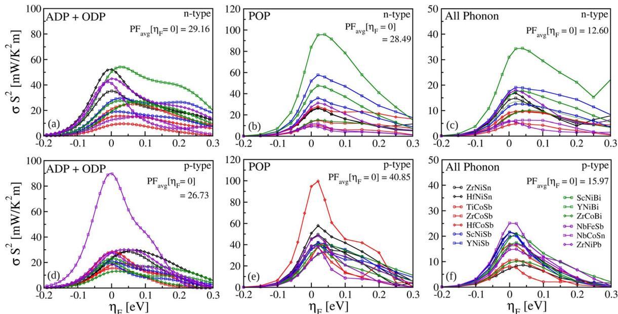
Fig. 4 The power factor *versus* density for all 13 HHs considered, for n-type (first row, a–c) and p-type (second row, d–f) polarities. The simulation results for three phonon scattering limited transport considerations are shown column-wise: (a and e) non-polar ADP + ODP scattering, (b and d) POP scattering, and (c and f) scattering due to all phonon processes combined (ADP + ODP + POP).
