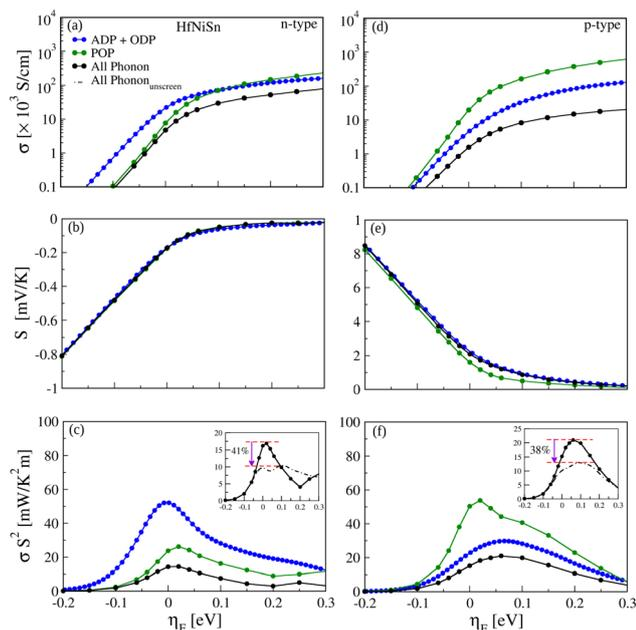
**Fig. 3** Thermoelectric coefficients for HfNiSn for n-type (left column) and p-type (right column) carriers. Three phonon scattering limited transport situations are presented: ADP + ODP, POP, and all phonon scattering. (a and d) Electrical conductivity. (b and e) Seebeck coefficient. (c and f) Power factor. Insets of (c) and (f): Comparison between the power factor computation results with (solid) and without (dashed) screening in the POP calculation.
